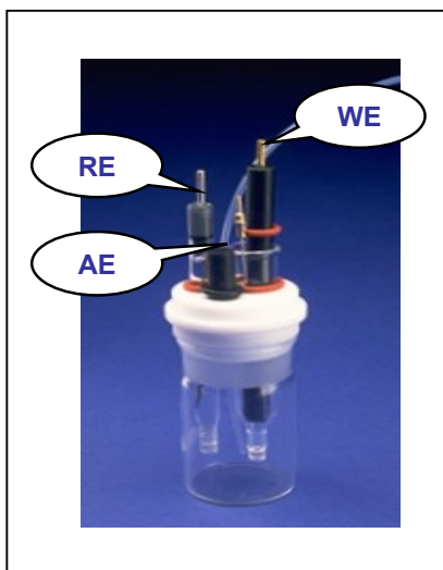
Figure 3. 2 A three electrode system electrochemical cell. WE = working electrode, RE = reference electrode and AE = auxiliary electrode
