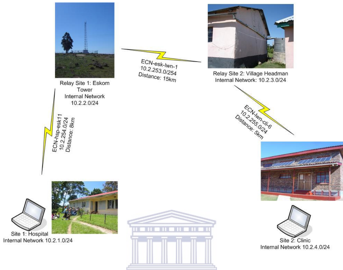
Figure 5.1: The network diagram: This diagram shows the structure of the network on which the MuTiv2 system runs. The network has two main sites and two relay points between the sites because of the long distances and lack of line of sight between the two main sites.
