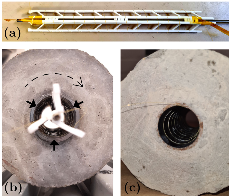
Fig. 5 Process of gluing the fibre on the internal surface of the hollow steel bar. a An optical fibre wound around the arms of the tool, restrained with tape. b Positioning of the fibre inside the hollow steel bar. The fibre obtained its helical shape by
