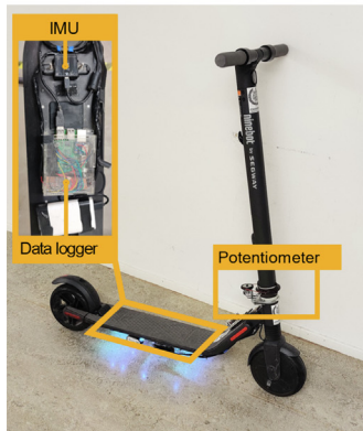
Fig. 1. Instrumented vehicles with data loggers and inertial measurement units (IMUs). Panels A. and B. are adapted from our previous work (Dozza et al., 2022).
