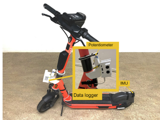
Fig. 1. Instrumented vehicles with data loggers and inertial measurement units (IMUs). Panels A. and B. are adapted from our previous work (Dozza et al., 2022).
