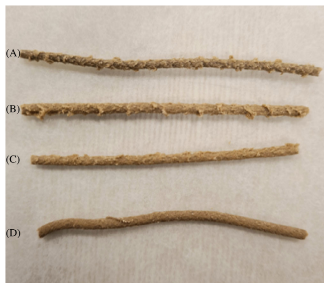
FIGURE 2 A visual impression of filaments composed of (A) PP-TMP, (B) PP-TMP AKD Hex, (C) PP-TMP AKD Lau, and (D) PP-TMP AKD St, as compounded for 10 min and extruded at 150 kN and 190°C.
