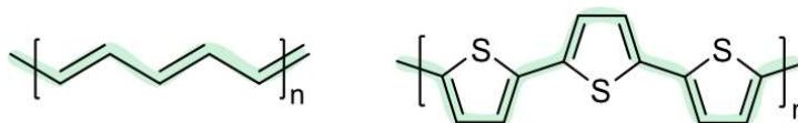
Figure 2.2. Chemical structure of conjugated polymers with the characteristic alternating single double carbon bonds.
