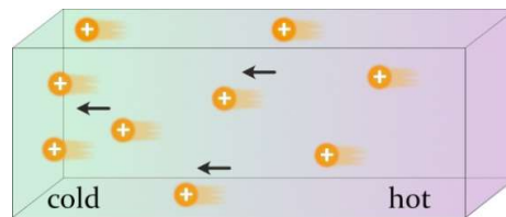
Figure 2.1. Thermoelectric effect in a p-type semiconductor.
