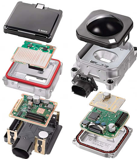
Figure 3.3: Exploded view of the Bosch RADAR sensors [71].
