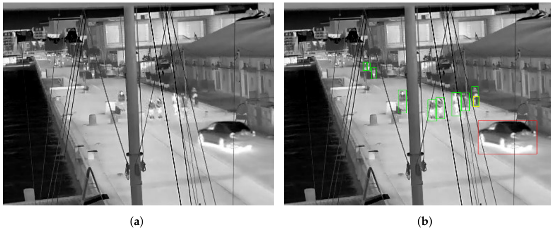
Figure A3. The example image used in Figures 10 and 11 is shown without bounding boxes (a) and with bounding boxes (b). In Figure 10 green, yellow, and red refer to person, bicycle, and vehicle classes, respectively.
