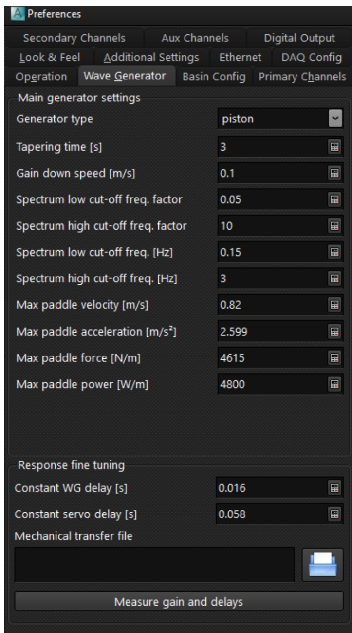
Figure 11. Screenshot from AwaSys wave generator software, showing the setting of a servo delay of 0.058 s (58 ms).
