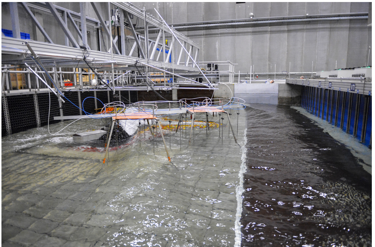
Testing of breakwater for Port of Hanstholm (19.01.2018).
