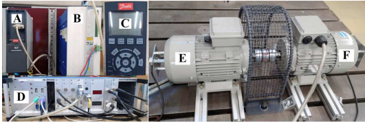
Fig. 7. Experimental Setup. (A) 3.0 kW Danfoss FC-302 inverter, (B) 14 kVA Servostar620 inverter, (C) Control panel (D) Self-made real-time controller (E) Main machine (F) Load machine.
