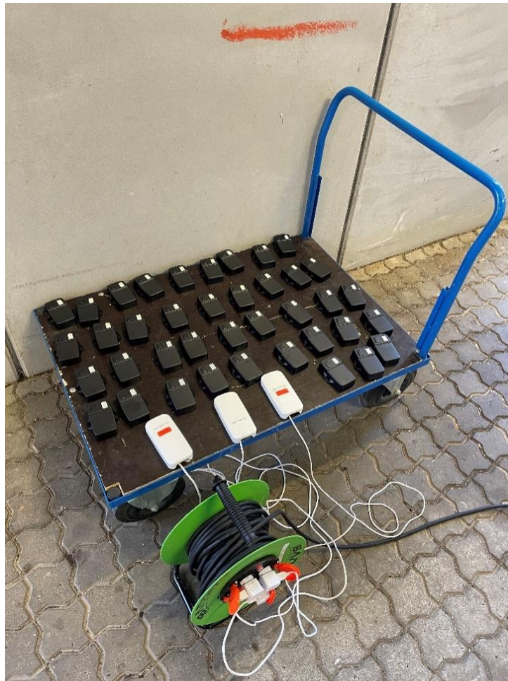
Figure 3: The IEQ sensors (black sensors) were tested and compared against IC meters (white sensors) under different conditions.
