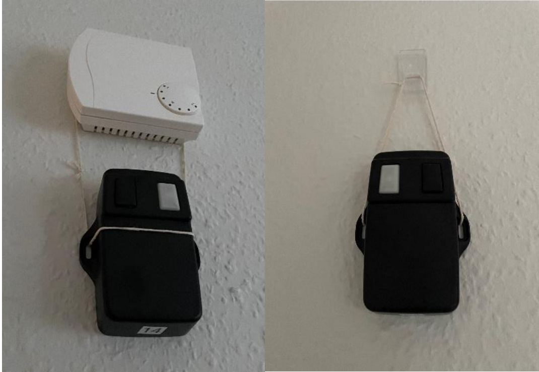
Figure 5: Installation of the IEQ sensors.
