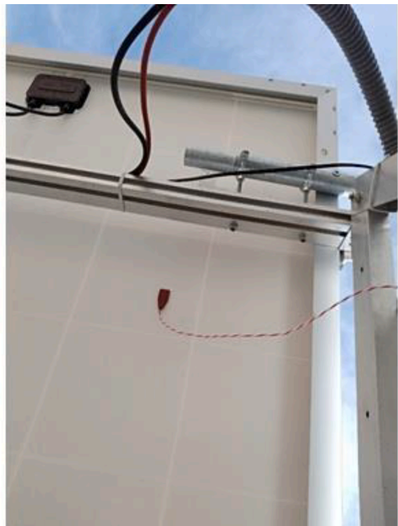
Fig. 11. Irradiance sensor (left) and panel temperature sensor (right) used to transmit weather data to the emulation in the RTDS in the tests performed.
