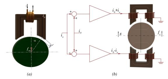
Figure 2. a) Radial single-pole active magnetic bearing; b) Differential control of one pair of poles of active magnetic bearing.
