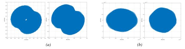
Figure 7. Graphic representation of the orbit - positions of the rotor axis in active magnetic bearings A and B; (a) without active control; (b) with active control.
