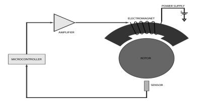
Figure 1. Schematic representation of the operation principle of a simple system of AMBs.
