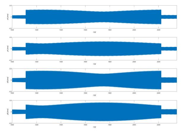
Figure 5. Graphic representation of rotor displacement along the x and y axes for AMBs A and B when during exploitation comes to the active control of the rigid rotor.
