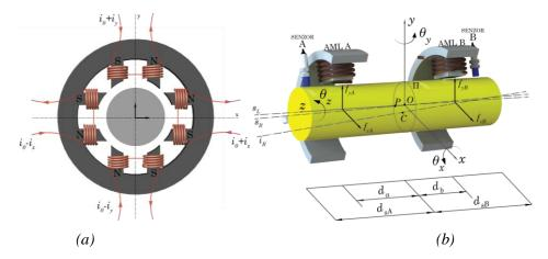
*Figure 3. (a) Structural configuration of an active magnetic bearing with two pairs of poles; (b) Structural model of the rotor system supported on two radial active magnetic bearings.*
