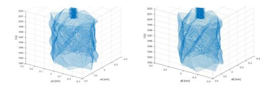
*Figure 6. Graphic representation of rotor displacement along the x and y axes for active magnetic bearings A and B when during exploitation comes to the active control of the rigid rotor.*
