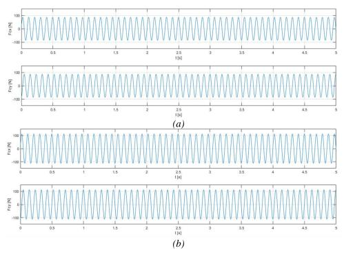
*Figure 8. Graphic representation of the centrifugal force caused by the unbalance in the x and y planes of the rigid rotor structure: (a) in the magnetic bearing A; (b) in magnetic bearing B.*
