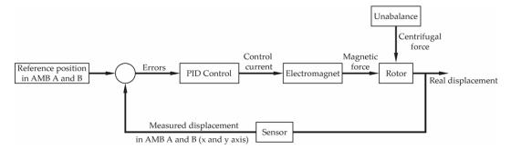
Figure 4. Block diagram of the AMB system control model.
