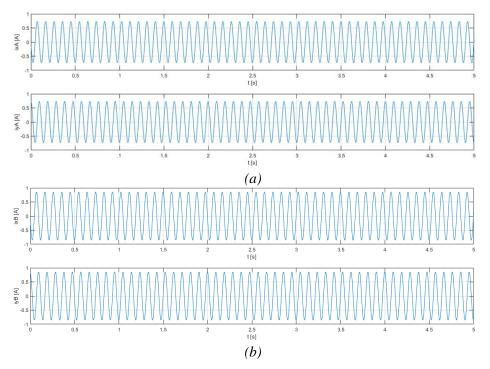
Figure 9. Graphical representation of the control currents required to position the rotor in the equilibrium position: (a) in the magnetic bearing A; (b) in magnetic bearing B.
