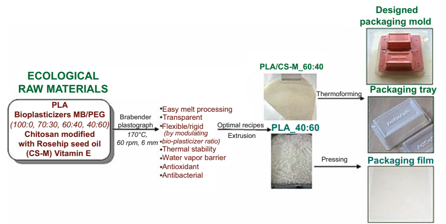
Fig. 12 Steps for obtaining food packaging system from biopolymers and blends (Darie-Niță et al. 2021)
