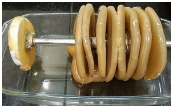
Fig. 8 BNC produced in advanced rotary disc bioreactor: BNC deposited on both sides of discs
