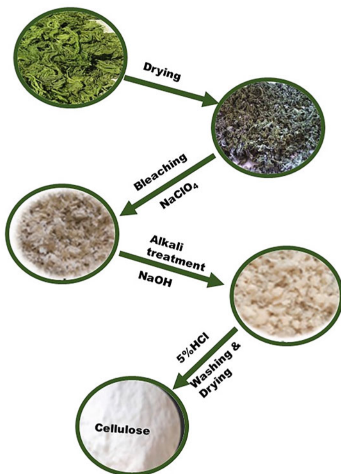
Fig. 3 Flow chart showing extraction of cellulose from Cladophora biomass
