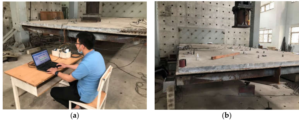
Figure 6. The process of measurement and sensor placement in one setup: (a) Data collection process; (b) Sensor placement in one setup.
