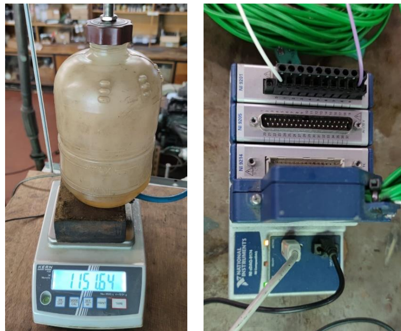
Figure 5. Fuel consumption measurement and data acquisition board.
