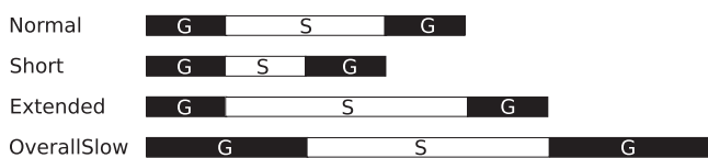
Fig. 6. Summary of the proportional timings for task execution. The grasp movement is depicted by “G” and the soldering process is depicted by “S”.
