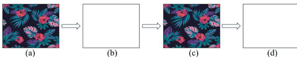
Figure 2. Operation scheme of reversible hydrochromic material: screen printed fabric (a); functionalization by the hydrochromic material (b); wetted fabric (c); dried fabric (d).
