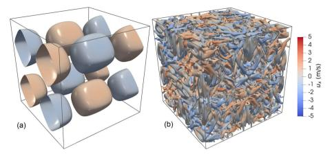
**Fig. 14** Visualization of the incompressible 3D Taylor-Green vortex from step 2 simulated with Open-FOAM showing iso-surfaces of the Q-criterion, colored by the *x*-component of velocity. At the beginning of the simulation, the flow is regular (**a**) but after some time decays into a pseudo-turbulence (**b**)
