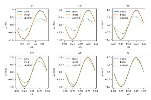
Fig. 29 Profiles of the x-component of velocity along the x-centerline at  $t/\tau_{ref} = 18$  for different mesh resolutions and discretization schemes
