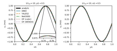
**Fig. 11** Velocity profiles along the centerlines of the computational domain at  $t = 10\tau_{ref}$  from the analytic solution, OpenFOAM (OF) and the three high-fidelity codes for the 2D TGV case from step 1
