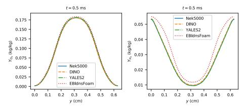
**Fig. 22** Profiles of  $O_2$  and  $H_2$  mass fractions along the *y* centerline at t = 0.5 ms for step 3. All simulations depicted here use the constant Lewis number diffusion approach
