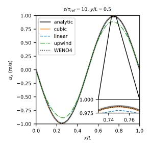
**Fig. 12** Velocity profile of  $u_x$  along the centerline at  $t = 10\tau_{ref}$  from OpenFOAM simulations with different spatial discretization schemes for the 2D TGV case from step 1
