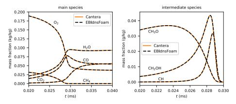
Fig. 7 Temporal evolution of species mass fractions of main (left) and intermediate (right) species for the auto-ignition case. The reference solution is provided by Cantera
