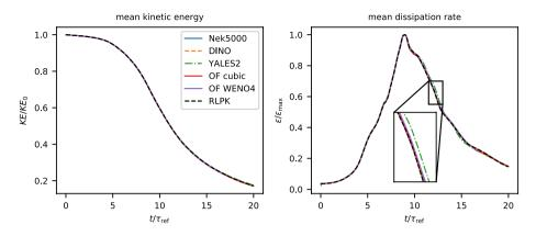
Fig. 16 Normalized volume-averaged kinetic energy (left) and dissipation rate (right) over time for the 3D incompressible TGV from step 2
