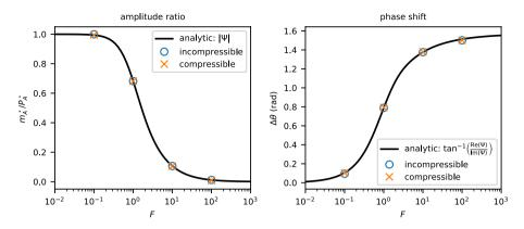
Fig. 5 Ratio of the normalized mass flow rate amplitude and normalized pressure gradient amplitude (left) as well as time shift between mass flow rate and pressure gradient (right) for pulsatile pipe flow
