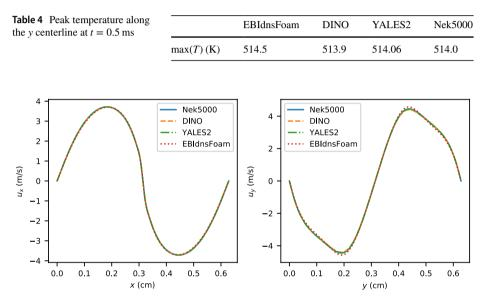
Fig. 21 Velocity profiles along the x and y centerlines at t = 0.5 ms for step 3
