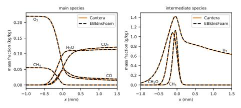
Fig. 9 Spatial profiles of species mass fractions of main (left) and intermediate (right) species for the freely propagating flame case. The reference solution is provided by Cantera
