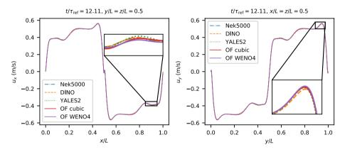
Fig. 15 Velocity profiles along the centerlines at  $t = 12.11\tau_{ref}$  for the 3D incompressible TGV from step 2
