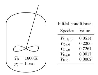
Fig. 6 Initial conditions for temperature T, pressure p and species mass fractions Y for the auto-ignition case
