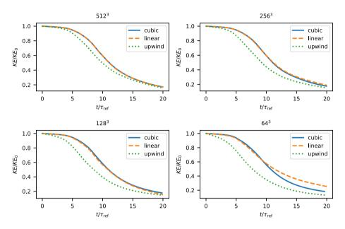
Fig. 30 Normalized volume-averaged kinetic energy over time for meshes with different mesh sizes, evaluated with the three standard OpenFOAM discretization schemes for the incompressible 3D TGV from Step 2
