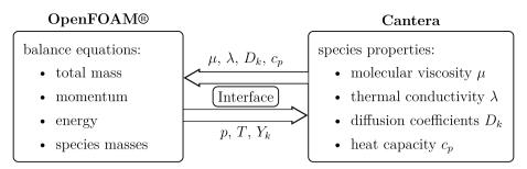
Fig. 1 Coupling between OpenFOAM and Cantera for the EBIdnsFoam code
