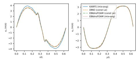
Fig. 26 Velocity profiles along the centerlines at t = 0.5 ms for step 4
