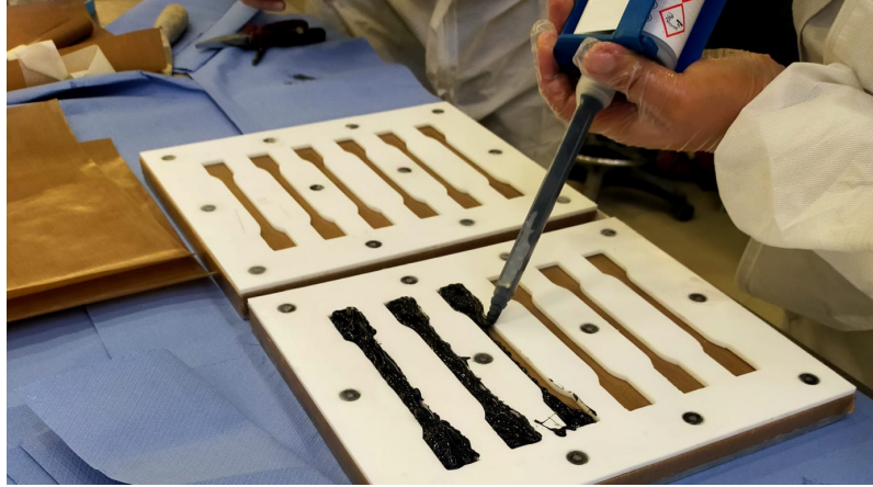
Figure 3.9: Application of the adhesive.
