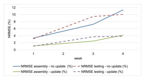
Figure 6-2 Development of the accuracy of the Digital Twin of line 1 with and without update
