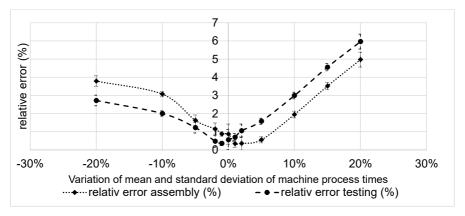
Figure 6-9 Change in relative error when varying mean and standard deviation including the 95% confidence interval
