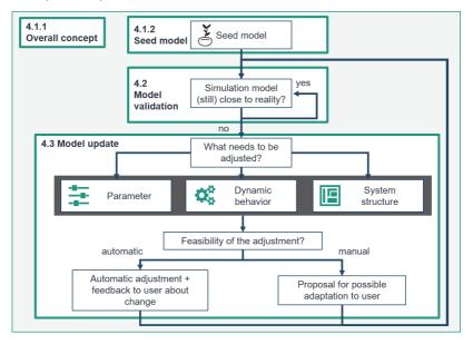
Figure 4-1 Function sketch of the Digital Twin of the production system including the respective text sections
