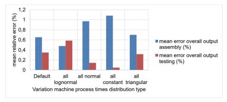
Figure 6-13 Change of relative error when changing distribution type
