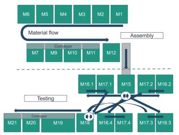
Figure 5-1 Schematic representation of the assembly and testing & completion subsystems
