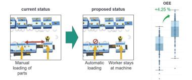
Figure 6-25 Example for the evaluation of hardware changes in the production system
