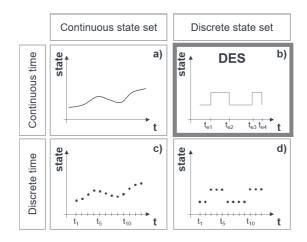
Figure 2-4 Classification of simulation models according to time and state set (Gutenschwager et al. 2017, p. 16) (based on Ören 1979, p. 36)
