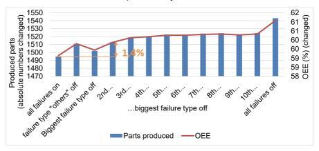
Figure 6-24 Influence of the most important failure types of machine 7 on the performance of the production system
