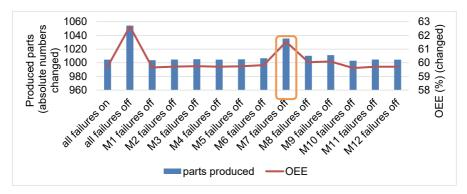
Figure 6-23 Influence of failures on different machines on the performance of the production system
