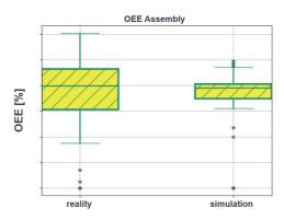
Figure 6-4 Boxplots of OEE per hour in reality and simulation
