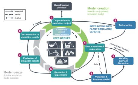
Figure 6-19 User concept Bosch use case (Overbeck et al. 2022)
