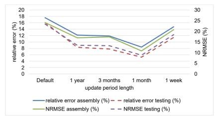
Figure 6-6 Accuracy with different update period lengths
