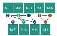
Figure 5-6 Example of employee loops in generic production area with machines A - I
