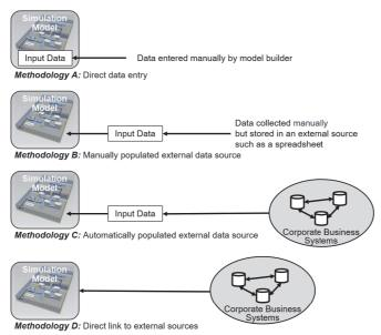
Figure 2-7 Ways to enter data into the simulation model (Robertson & Perera 2002)
