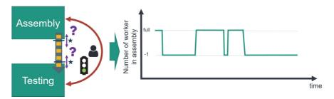
Figure 6-21 Determination of threshold to inform worker when to change subsystem
