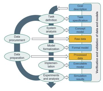
Figure 2-6 Procedure model for simulation projects according to VDI (2014)
