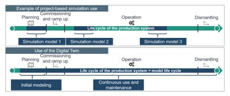
Figure 1-1 Use of conventional simulation models versus the use of a Digital Twin
