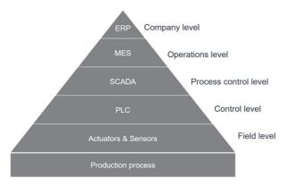
Figure 2-12 The automation pyramid (Siepmann 2016)
