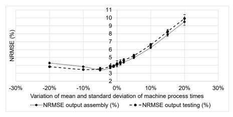
Figure 6-10 Change of NRMSE when varying mean and standard deviation including the 95% confidence interval (Overbeck et al. 2023)
