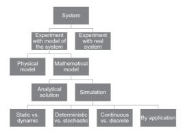
Figure 2-3 Ways to examine a system (based on Law (2015, p. 4))
