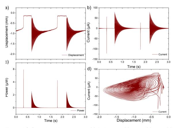
**Figure 21** Self-actuation without resonance, (a) displacement, (b) current, (c) power, (d) plotting displacement vs current to check cyclic behavior.
