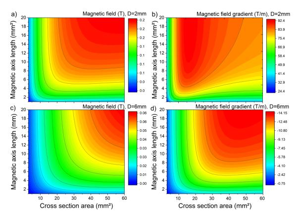
**Figure 58** LEM simulation of the effect of dimensions of magnet, (a) magnetic field at a distance (D) of 2 mm from magnet surface, (b) magnetic field gradient at D = 2 mm, (c) magnetic field at D = 6 mm, (d) magnetic field gradient at D = 6 mm.
