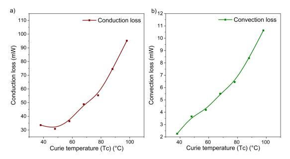
**Figure 74** LEM simulation of effect on loss mechanisms of the TMG with 10  $\mu$ m Ni-Mn-Ga film, (a) conduction losses, (b) convection losses.
