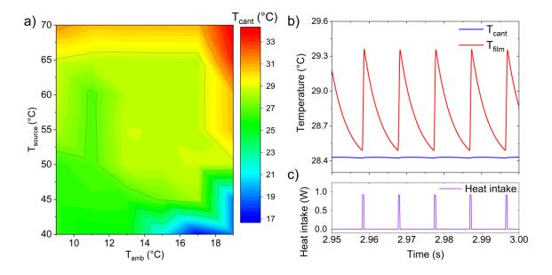
**Figure 98** (a) temperature of the cantilever (b) Temperature profile of the TMG layers. Reprinted from Joseph et al.<sup>152</sup>
