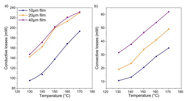
**Figure 78** LEM simulation of the effect of thickness on losses, (a) conduction losses, (b) convection losses. Data pre-published in Joseph et al.<sup>28</sup>
