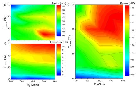
**Figure A 11** The mechanical and electrical performance of the Gd TMG device as a function of load resistance ( $R_L$ ) and heat source temperature ( $T_{source}$ ) at 13 °C ambient temperature were investigated. The supplied color code can be used to calculate numerical values. (a) Cantilever front stroke during resonant self-actuation, (b) cantilever front oscillation frequency, (c) electrical power output determined from the induced current of the pick-up coil.
