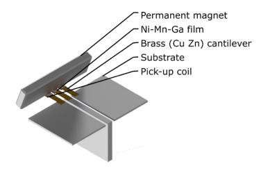
**Figure 87** Parallelization with three devices, with the substrate for the center device rotated by 90° to allow low separation between devices.
