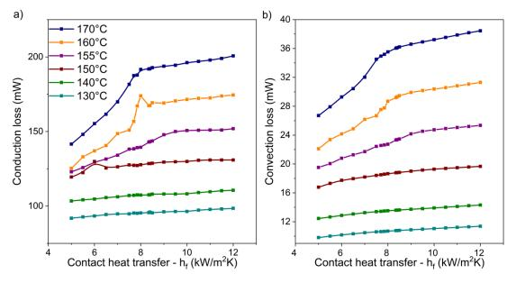
Figure 61 LEM simulation of the TMG with 10 μm Ni-Mn-Ga film, (a) conduction losses,
