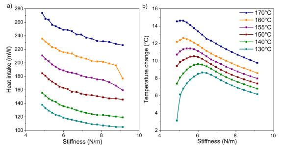
**Figure 66** LEM simulation of the effect of cantilever stiffness on (a) heat intake and (b)  $\Delta T$  within the TM film of the TMG with 10 µm Ni-Mn-Ga film. Legend shown is T<sub>source</sub>.
