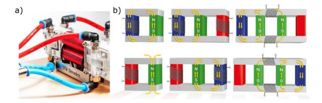
**Figure 29** Thermomagnetic generator with a pretzel-like magnetic topology introduced in Waske et al.,<sup>110</sup> (b) image of the TMG prototype, (b) different topology of magnetic circuits discussed. Reprinted with permission from Springer Nature.
