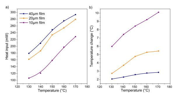
**Figure 77** LEM simulation of the effect of film thickness on (a) heat intake and (b) the average temperature change within the TM film. Data pre-published in Joseph et al.<sup>28</sup>
