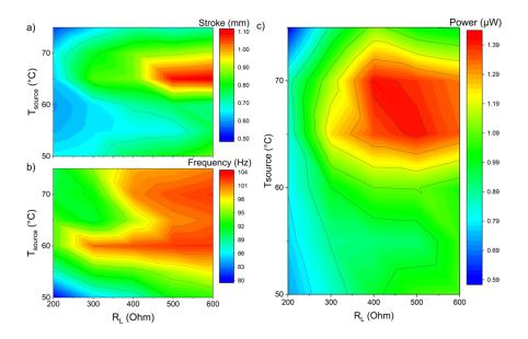
**Figure A 8** The mechanical and electrical performance of the Gd TMG device as a function of load resistance ( $R_L$ ) and heat source temperature ( $T_{source}$ ) at 19 °C ambient temperature were investigated. The supplied color code can be used to calculate numerical values. (a) Cantilever front stroke during resonant self-actuation, (b) cantilever front oscillation frequency, (c) electrical power output determined from the induced current of the pick-up coil.
