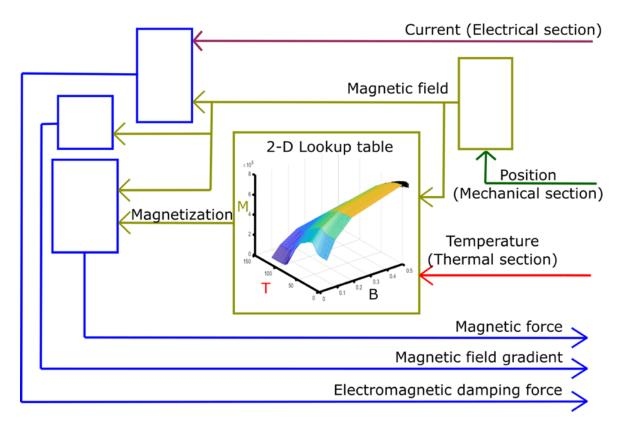
**Figure 40** Magnetic Section with the temperature of the TM film and position of the beam front as inputs. The magnetic force, magnetic field gradient, and electromagnetic damping force are the outputs of the section. Reprinted from Joseph et al.<sup>128</sup>
