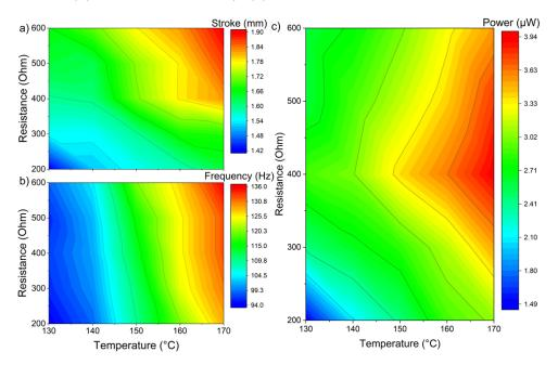
**Figure A 3** The mechanical and electrical performance of the TMG device with Ni-Mn-Ga 20 $\mu$ m as a function of load resistance (R<sub>L</sub>) and heat source temperature (T<sub>source</sub>). The supplied color code can be used to calculate numerical values. (a) Stroke during resonant self-actuation, (b) oscillation frequency, (c) electrical power output.
