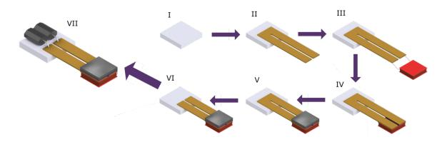
**Figure 93** Fabrication steps involved in the preparation of a TMG with Gadolinium as the TM active material. Adapted image from Joseph et al.<sup>152</sup>
