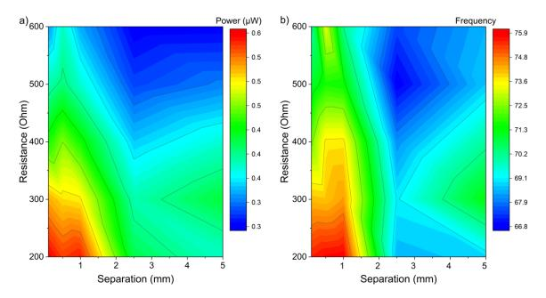
**Figure A 6** Effect of resistance and separation on performance of TMG in three device array with 20µm Ni-Mn-Ga film. (a) Power output of TMG, (b) frequency of TMG operation.
