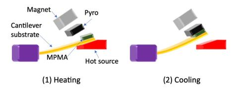
**Figure 33** The schematic of the TMG with a pyroelectric element for energy conversion directly from heat to electricity.<sup>117</sup> Reprinted with permission from Applied Energy.
