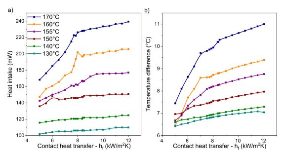
**Figure 60** LEM simulation of the TMG with 10  $\mu$ m Ni-Mn-Ga film, (a) Heat intake into film, and (b) temperature change ( $\Delta$ T) within the film. Legend shown is T<sub>source</sub>. Data pre-published in Joseph et al.<sup>91</sup>
