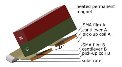
**Figure 81** Schematic of two TMG's operating in parallel under a long magnet. Adapted from Joseph et al.<sup>150</sup>
