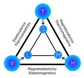
Figure 2 Mechanical, magnetic, and thermal coupling in multiferroic materials.<sup>52</sup>
