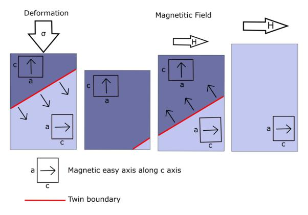
**Figure 6** Schematic diagram of the tetragonal structure of Ni-Mn-Ga single crystal showing reorientation.<sup>3</sup>
