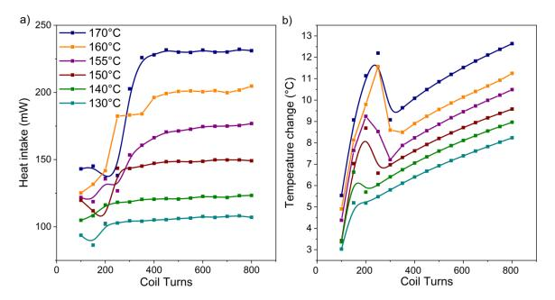
**Figure 69** LEM simulation of the effect of pick-up coil on (a) heat intake and (b) temperature change within the material of the TMG with 10  $\mu$ m Ni-Mn-Ga film. Legend shown is T<sub>source</sub>.
