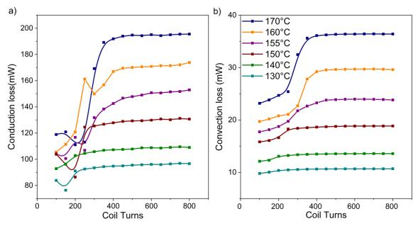
Figure 70 LEM simulation of the effect of pick-up coil turns on heat dissipation of the TMG with 10  $\mu$ m Ni-Mn-Ga film, (a) conduction losses, (b) convection losses. Legend shown is T<sub>source</sub>.
