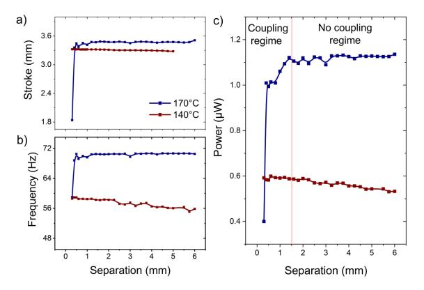
**Figure 83** Effect of separation on the TMG at  $T_{source}$  of 170 °C and 140 °C. (a) Stroke of the deflection of the TMG, (b) Frequency of operation of the TMG, (c) power output of the TMG. Part of data pre-published in Joseph et al.<sup>150</sup>
