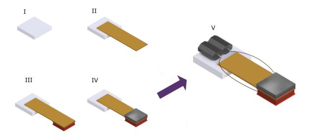
Figure 47 Fabrication steps for preparing a TMG prototype.
