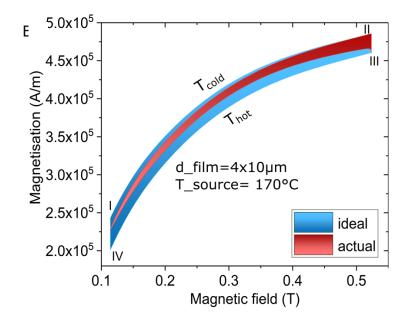
**Figure A 1** The magnetization cycle in TMG, with values corresponding to operation in resonant self-actuation mode of TMG with  $40\mu$ m Ni-Mn-Ga film. Adapted from Joseph et al.<sup>28</sup>
