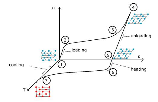
**Figure 4** Shape memory effect, the stress-strain-temperature diagram of the one-way effect of shape memory alloys (SMAs).<sup>63</sup>
