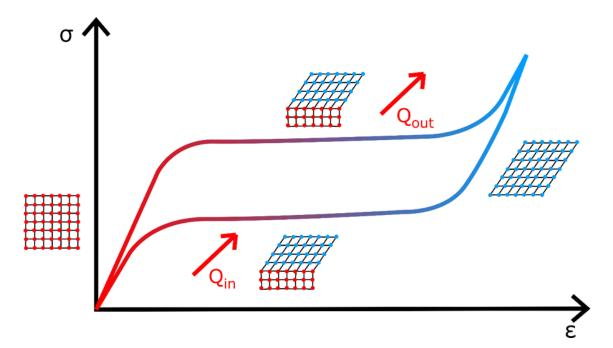
Figure 5 SMA superelastic effect stress-strain characteristics.<sup>64</sup>
