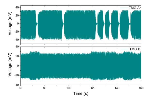
**Figure 86** Simultaneous performance comparison of the TMG devices. The  $T_{source}$  is maintained at 170 °C and separation is 1000 µm, (a) voltage output across load resistance for TMG sample A, (b) voltage across load resistance for TMG sample B. Data pre-published in Joseph et al.<sup>150</sup>
