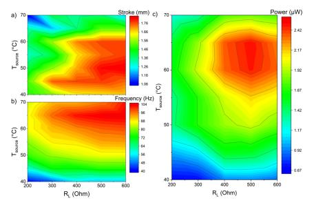
**Figure A 12** The mechanical and electrical performance of the Gd TMG device as a function of load resistance ( $R_L$ ) and heat source temperature ( $T_{source}$ ) at 9 °C ambient temperature were investigated. The supplied color code can be used to calculate numerical values. (a) Cantilever front stroke during resonant self-actuation, (b) cantilever front oscillation frequency, (c) electrical power output determined from the induced current of the pick-up coil.
