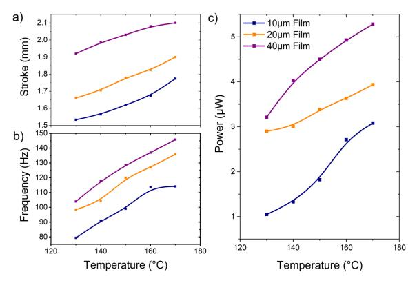
**Figure 76** Effect of film thickness on the performance of the device, (a) stroke, (b) frequency, (c) power output. Data pre-published in Joseph et al.<sup>28</sup>
