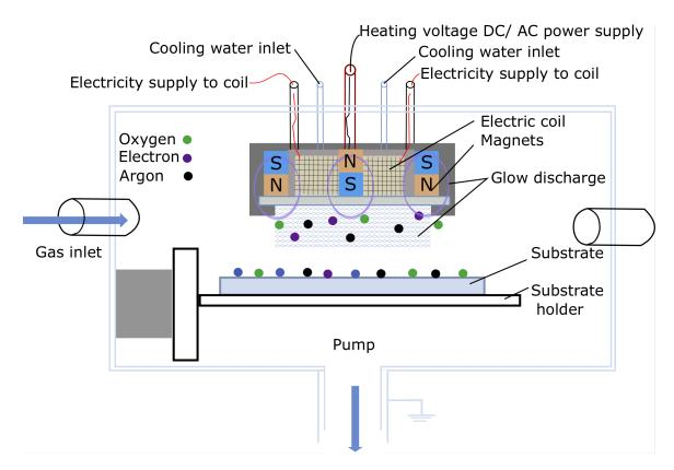
Figure 11 Schematic of Magnetron Sputtering. Adapted from Hassan et al.<sup>81</sup> 26
