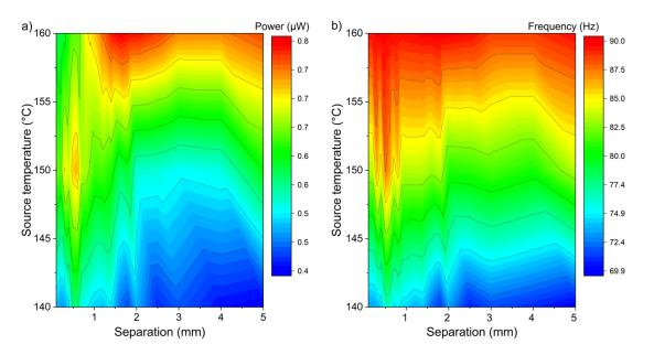
**Figure 89** Performance of center device in the TMG array of three devices with 20  $\mu$ m Ni-Mn-Ga film, (a) power output, (b) frequency of operation.
