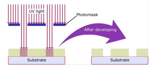
Figure 14 Schematic using UV lithography.
