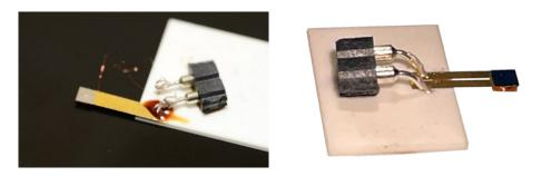
**Figure 92** (a) Device with overhanging copper wires from pick-up coil attached to the connector (b) TMG with double beam brass cantilever as electrodes with no overhang. Adapted image from Joseph et al.<sup>152</sup>
