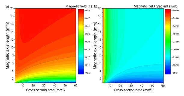
**Figure 57** LEM simulation of the effect of dimensions of magnet on (a) magnetic field, and (b) magnetic field gradient, at the surface of the magnet.
