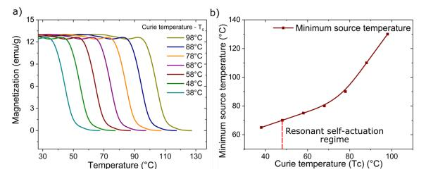
**Figure 71** (a) LEM simulated values of magnetization vs temperature characteristics shifted for decreasing Curie temperature ( $T_c$ ), (b) LEM simulation of minimum  $T_{source}$  for different values of  $T_c$ . Part of data pre-published in Joseph et al.<sup>128</sup>
