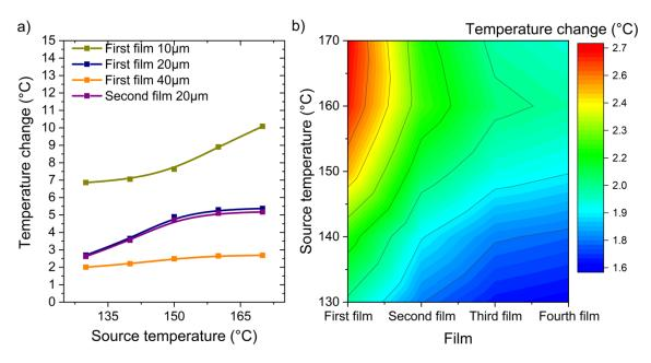
**Figure 79** LEM simulation of (a) temperature change within different film layers in a TM film stack (b) temperature profile within the TM film stack in a TMG with 4 films (40  $\mu$ m effective thickness). Part of data pre-published in Joseph et al.<sup>28</sup>
