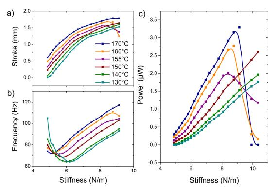
**Figure 65** LEM simulation of the effect of cantilever stiffness on the performance of the TMG with 10  $\mu$ m Ni-Mn-Ga film, (a) stroke of deflection, (b) frequency of operation, (c) power output. Legend shown is T<sub>source</sub>.
