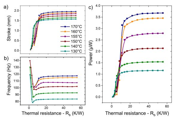
**Figure 62** LEM simulation of  $R_b$  on the performance of a TMG with 10 µm Ni-Mn-Ga film, (a) stroke, (b) frequency, (c) power output. Legend shown is  $T_{source}$ . Data pre-published Joseph et al. <sup>91</sup>
