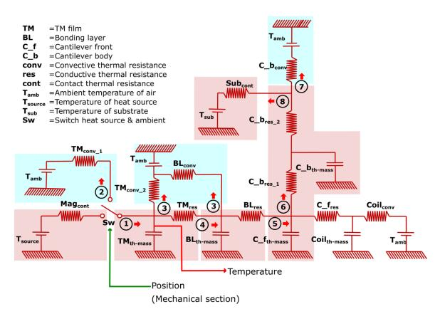
**Figure 42** LEM of thermal section takes in position as input and generates the temperature of different components (like film, cantilever, etc.) as the outputs. Reprinted from Joseph et al.<sup>91</sup>
