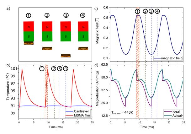
**Figure 50** (a) Device operating stages (b) temperature change within Ni-Mn-Ga film, (c) magnetic field change, (d) magnetization change in the Ni-Mn-Ga film. Reprinted from Joseph et al. <sup>128</sup>
