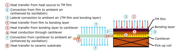
Figure 41 Heat transfer processes in the TMG assembly. Reprinted from Joseph et al.<sup>91</sup>
