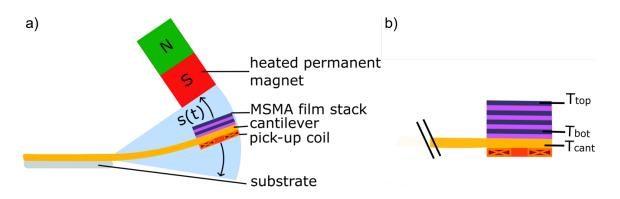
**Figure 75** Design of film stack to increase the thickness (a) schematic of the TMG with oscillating cantilever and Ni-Mn-Ga film stack, (b) section of the cantilever front showing the film stack with multiple layers of Ni-Mn-Ga films. Adapted from Joseph et al.<sup>28</sup>
