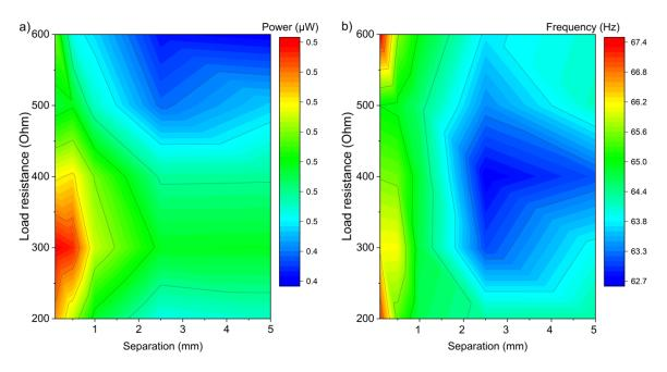
**Figure A 5** Effect of resistance and separation on performance of TMG at center in three device array with 10µm Ni-Mn-Ga. (a) Power output of TMG, (b) frequency of operation of TMG.
