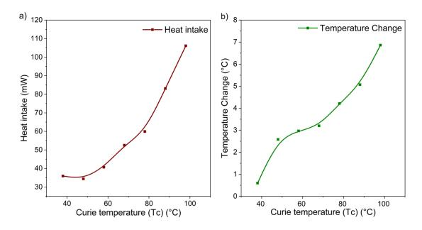
**Figure 73** LEM simulation of the effect of curie temperature ( $T_c$ ) on the TMG with 10  $\mu$ m Ni-Mn-Ga film (a) heat intake and (b) temperature change in the TM film.
