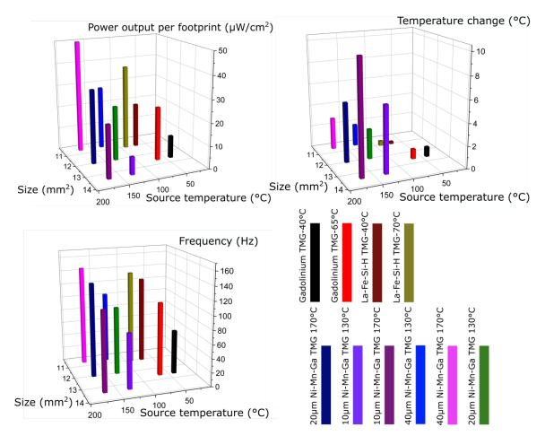
**Figure 103** Comparison of thermomagnetic generators presented as part of this work (a) power per footprint of devices, (b) temperature change within active material of the device, (c) frequency of operation of the devices.
