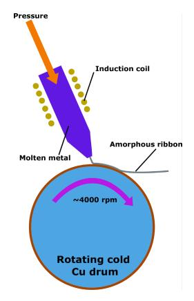
Figure 12 Schematic of fabrication by melt spinning.
