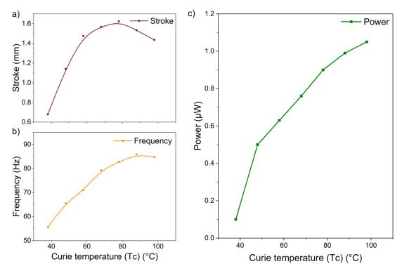
**Figure 72** LEM simulation of the effect of Tc on the performance of the TMG with 10  $\mu$ m Ni-Mn-Ga film at minimum source temperature, (a) stroke, (b) frequency, (c) power output.
