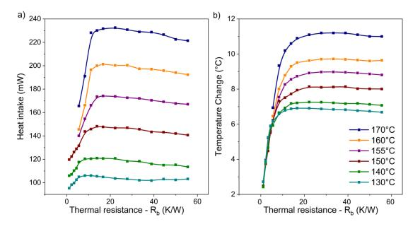
**Figure 63** LEM simulation of the effect of  $R_b$  on the TMG with 10 µm Ni-Mn-Ga film, (a) heat intake at contact, and (b) temperature change within the TM film. Legend shown is  $T_{source}$ . Data pre-published in Joseph et al.<sup>91</sup>
