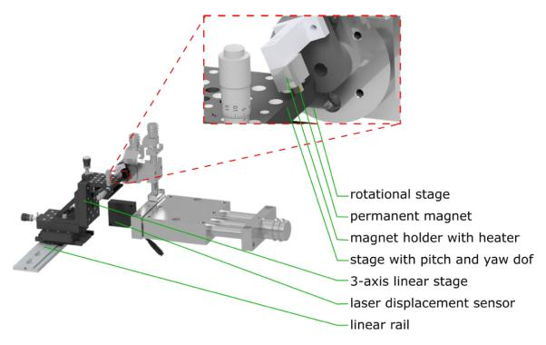
**Figure 45** 3D model of the experimental setup used to measure the output of the thermomagnetic generators, allowing for several degrees of freedom.
