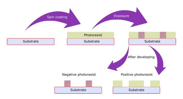
Figure 13 Schematic of fabrication using a lithography process.
