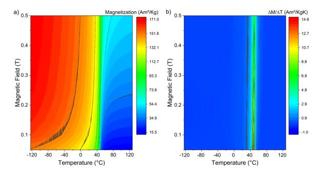
**Figure 99** (a)Magnetization measurement for the La-Fe-Si-H sample, (b)  $\Delta M/\Delta T$  for La-Fe-Si-H sample with respect to changing temperature.
