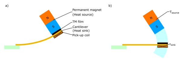
**Figure 19** Schematic of the thermomagnetic generator self-actuation (a) heating at contact with the permanent magnet as the heat source, (b) cooling during the self-actuation. Reprinted from Joseph et al.<sup>91</sup>
