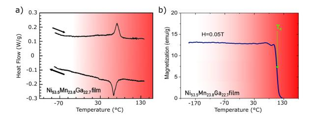
**Figure 46** (a) DSC measurement of Ni-Mn-Ga alloy (b) Magnetization measurement for varying temperatures for Ni-Mn-Ga film. Reprinted from Joseph et al.<sup>28</sup>
