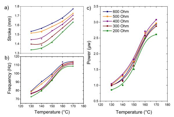
**Figure 48** Effect of  $R_L$  on the performance of the TMG (a) stroke of deflection, (b) frequency of oscillation, (c) power output from the pick-up coil. Part of data pre-published in Joseph et al.<sup>28,91,128</sup>
