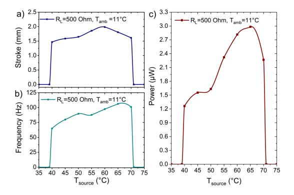
**Figure 94** Mechanical and electrical performance of the Gd-film TMG as a function of heat source temperature ( $T_{source}$ ) at 11 °C ambient temperature: a) Cantilever-front stroke during resonant self-actuation, b) cantilever oscillation frequency, c) electrical power output at a load resistance of 500 Ohm. Data pre-published in Joseph et al.<sup>152</sup>
