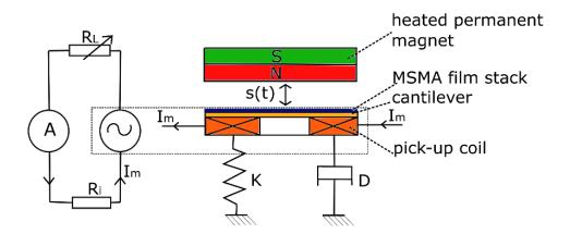
**Figure 44** Electromechanical circuit diagram of a TMG. A spring-mass-damper system with stiffness K and damping constant D make up the mechanical component. The pick-up coil's internal resistance ( $R_i$ ) and the  $R_L$  are both included in the electrical component. I<sub>m</sub> stands for the induced electrical current. Adapted from Joseph et al.<sup>28</sup>
