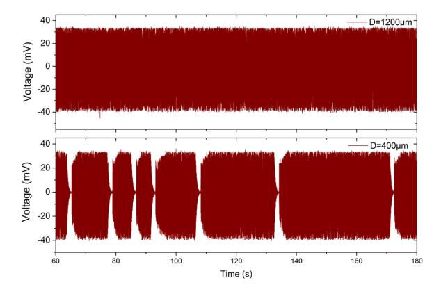
**Figure 85** Output performance of the TMG (a) at a separation of 1200  $\mu$ m between devices and (b) 400  $\mu$ m between devices. Data pre-published in Joseph et al.<sup>150</sup>
