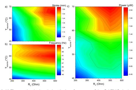
**Figure A 10** The mechanical and electrical performance of the Gd TMG device as a function of load resistance ( $R_L$ ) and heat source temperature ( $T_{source}$ ) at 15 °C ambient temperature were investigated. The supplied color code can be used to calculate numerical values. (a) Cantilever front stroke during resonant self-actuation, (b) cantilever front oscillation frequency, (c) electrical power output determined from the induced current of the pickup coil.
