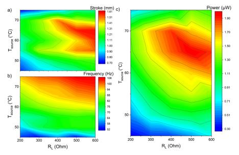
**Figure A 9** The mechanical and electrical performance of the Gd TMG device as a function of load resistance ( $R_L$ ) and heat source temperature ( $T_{source}$ ) at 17°C ambient temperature were investigated. The supplied color code can be used to calculate numerical values. (a) Cantilever front stroke during resonant self-actuation, (b) cantilever front oscillation frequency, (c) electrical power output determined from the induced current of the pick-up coil.
