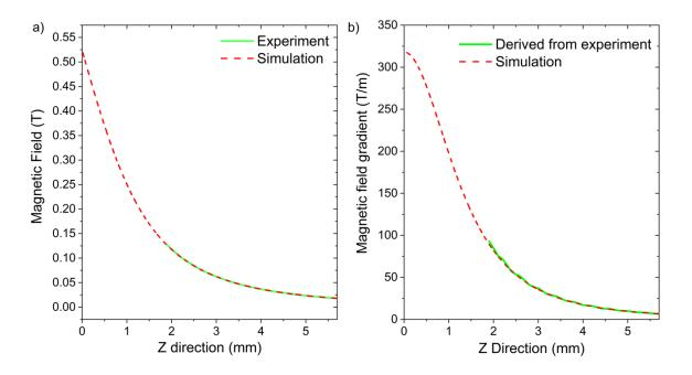
**Figure 56** Direct comparison of magnetic field measurements and magnetic field simulation. (a) Magnetic field along the z direction at the center determined by measurement and simulation, (b) magnetic field gradient derived from magnetic field measurement and simulation along the z direction at the center.
