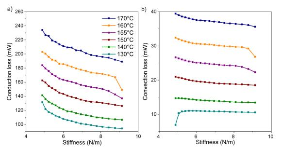
**Figure 67** LEM simulation of the effect of stiffness, (a) conduction losses, (b) convection losses. Legend shown is  $T_{source}$ .
