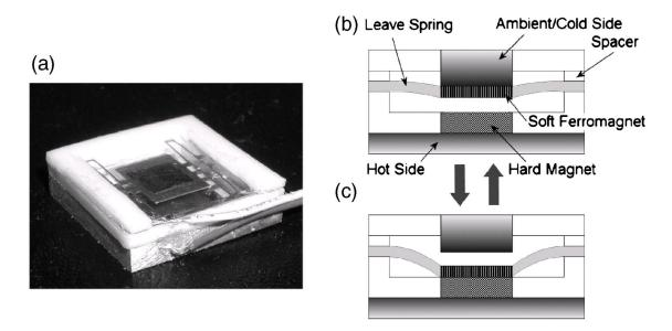
**Figure 30** TMG using ferromagnetic Gadolinium as active material presented in, (a) actuation device, (b) cross-sectional view during cooling, (c) cross-sectional view during heating.<sup>111</sup> Reprinted with permission from AIP publishing.
