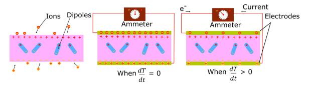
Figure 9 Schematic of pyroelectric effect. Adapted from Whatmore et al. <sup>73</sup>
