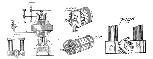
Figure 23 Pyromagnetic motor from US patent 380100 by Thomas Edison<sup>96</sup>
