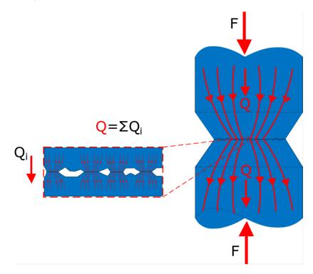
**Figure 10** Contact heat transfer between the solid surfaces in contact. Adapted from Wang et al.<sup>78</sup>
