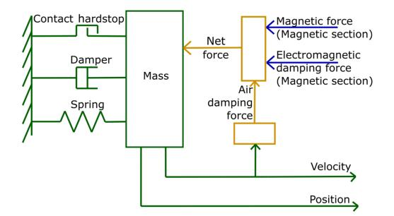
**Figure 39** Mechanical section with inputs of magnetic force and electromagnetic damping force and outputs of velocity and position of the beam front. Reprinted from Joseph et al.<sup>128</sup>
