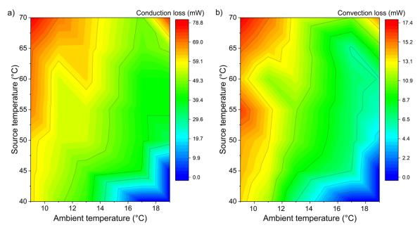
**Figure 97** LEM simulation of the effect of ambient temperature on the loss mechanism (a) conduction losses from the Gadolinium film into the cantilever, (b) convection losses into the ambient air from the Gadolinium film. Reprinted from Joseph et al.<sup>152</sup>
