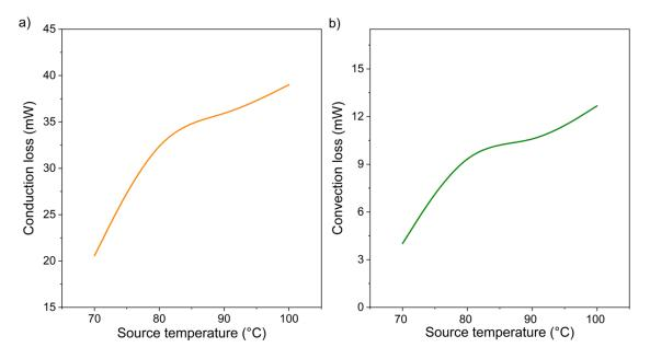
Figure 102 LEM simulation of thermal losses, (a) conduction losses from the La-Fe-Si film to the cantilever through the  $R_b$ , (b) convection losses from the film directly to the ambient. 146
