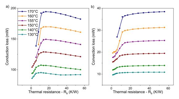
**Figure 64** LEM simulation of the effect of  $R_b$  on heat dissipation in the TMG with 10 µm Ni-Mn-Ga film, (a) conduction losses, (b) convection losses. Legend shown is  $T_{source}$ . Part of data pre-published in Joseph et al.<sup>91</sup>
