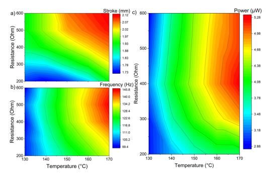
**Figure A 4** The mechanical and electrical performance of the TMG device with Ni-Mn-Ga 40 $\mu$ m as a function of load resistance (R<sub>L</sub>) and heat source temperature (T<sub>source</sub>). The supplied color code can be used to calculate numerical values. (a) Stroke during resonant self-actuation, (b) oscillation frequency, (c) electrical power output.
