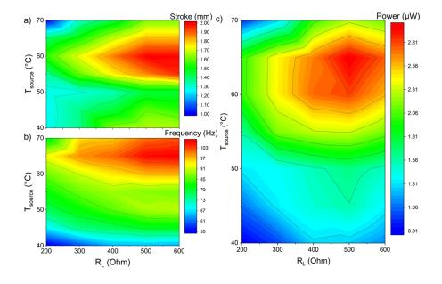
**Figure A 7** The mechanical and electrical performance of the Gd TMG device as a function of load resistance ( $R_L$ ) and heat source temperature ( $T_{source}$ ) at 11 °C ambient temperature were investigated. The supplied color code can be used to calculate numerical values. (a) Cantilever front stroke during resonant self-actuation, (b) cantilever front oscillation frequency, (c) electrical power output.
