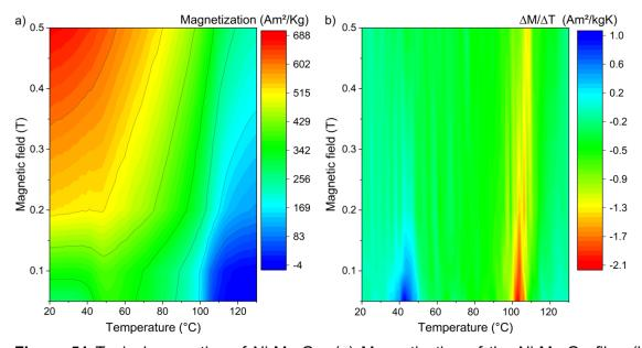
**Figure 51** Typical properties of Ni-Mn-Ga. (a) Magnetization of the Ni-Mn-Ga film, (b)  $\Delta M/\Delta T$  derived from magnetization to observe the change in magnetization with respect to temperature change. The data for this graph was extracted from Gueltig et al.<sup>92</sup>
