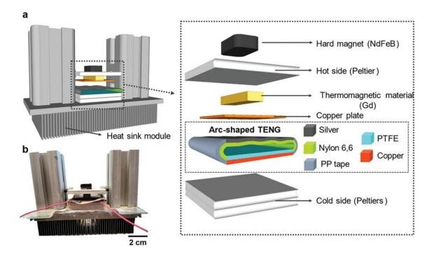
Figure 32 Hybrid thermomagnetic and triboelectric nanogenerator presented in Ahmim et al.<sup>115</sup> Reprinted with permission from John Wiley and Sons. Legend: TENG- triboelectric nanogenerator, PP tape- polypropylene tape, PTFE- polytetrafluoroethylene.
