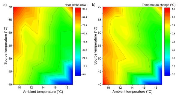
**Figure 96** LEM simulation of the effect of ambient temperature on thermal performance (a) average heat intake into the Gadolinium film on contact, (b) average temperature change of the Gadolinium film. Reprinted from Joseph et al.<sup>152</sup>
