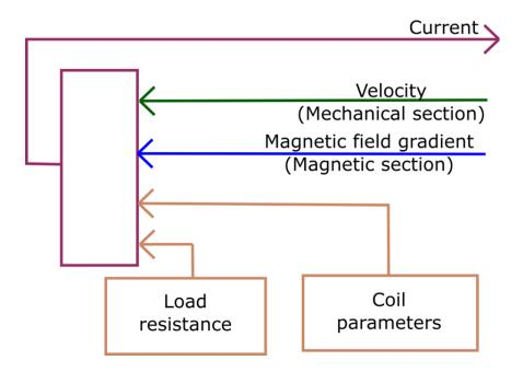
**Figure 43** Electrical section takes in the velocity of the beam front and magnetic field gradient as the input to the section and generated current is given out as output. Pick-up coil parameters and  $R_L$  do not change during the simulation of one configuration and hence are given as constants. Reprinted from Joseph et al.<sup>128</sup>
