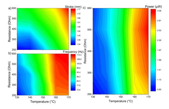
**Figure A 2** The mechanical and electrical performance of the TMG device with Ni-Mn-Ga 10 $\mu$ m as a function of load resistance (R<sub>L</sub>) and heat source temperature (T<sub>source</sub>). The supplied color code can be used to calculate numerical values. (a) Stroke during resonant self-actuation, (b) oscillation frequency, (c) electrical power output.
