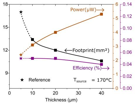
Figure 80 Effect of scaling on power, footprint, and efficiency. Adapted from Joseph et al.<sup>28</sup> 114
