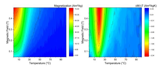
**Figure 90** (a)Magnetization measurement taken by varying temperature at different magnetic fields (b) Magnetization gradient, derived from the magnetization measurement. Data is pre-published in Joseph et al.<sup>152</sup>
