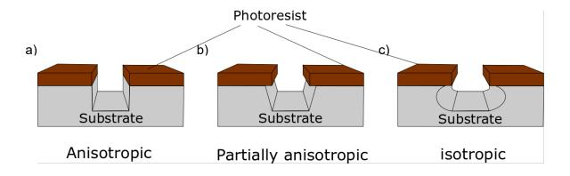
**Figure 16** Schematic of various wet etching processes (a) anisotropic etching, (b) partially anisotropic, (c) isotropic etching.
