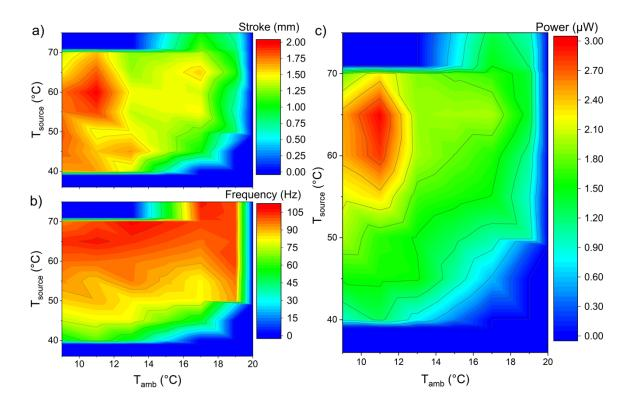
Figure 95 Effect of ambient temperature on the performance of the device, (a) stroke of cantilever deflection, (b) frequency of cantilever oscillation, (c) power output. Reprinted from Joseph et al.<sup>152</sup>
