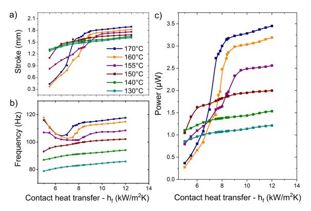
**Figure 59** LEM simulation of the effect of Contact heat transfer coefficient ( $h_f$ ) on the performance of the TMG with 10 µm Ni-Mn-Ga film, (a) stroke of the cantilever deflection, (b) frequency of oscillation of cantilever, (c) power output from the pick-up coil. Legend shown is T<sub>source</sub>. Data pre-published in Joseph et al.<sup>91</sup>
