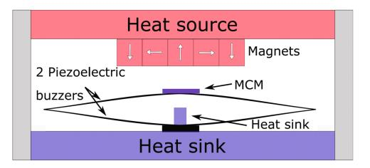
**Figure 31** Schematic of the TMG with La-Fe-Si as active material and piezo spring as energy transducing material.<sup>114</sup> Reprinted with permission from Elsevier.
