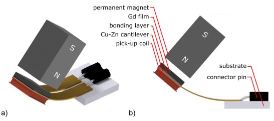
**Figure 91** (a) 3D schematic of the double beam TMG with Gadolinium film at the tip, (b) side view of the TMG showing the component names. Adapted image from Joseph et al.<sup>152</sup>
