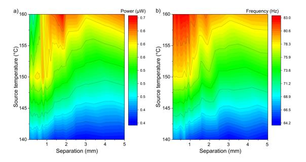
**Figure 88** Performance of the center device (the TMG with 10  $\mu$ m Ni-Mn-Ga film) in an array of three devices as the separation is gradually reduced. The two neighboring devices are moved and kept at the same separation. (a) power output of the TMG (b) frequency of the TMG.
