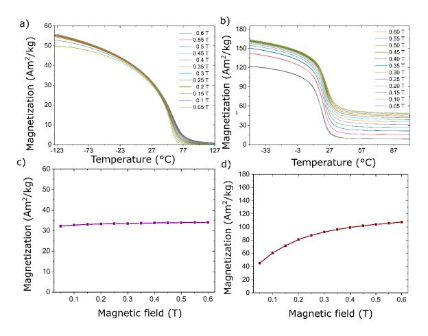
**Figure 18** (a) Magnetization vs temperature graph for a Ni-Mn-Ga alloy. (b) Magnetization vs temperature graph for a La-Fe-Si-Mn-H alloy (c) Magnetization vs magnetic field for Ni-Mn-Ga alloy at room temperature (d) Magnetization vs magnetic field for La-Fe-Si-Mn-H at room temperature.
