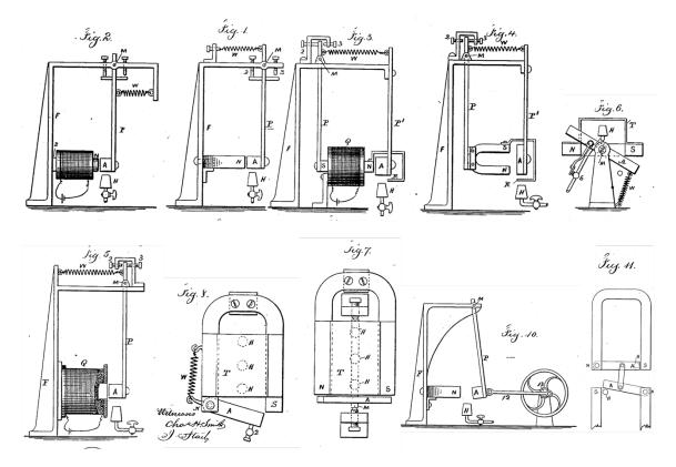
Figure 24 Designs of the thermomagnetic motor by Nikola Tesla in US patent 39612197
