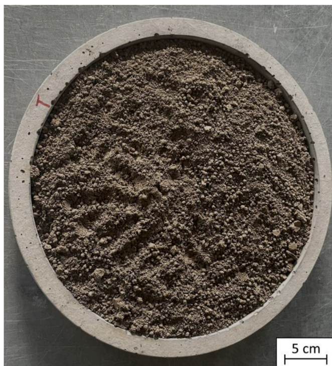
Fig. 3. Pre-sintered granulates with 60 vol% 316 L and 40 vol% carbonless MgO powder.
