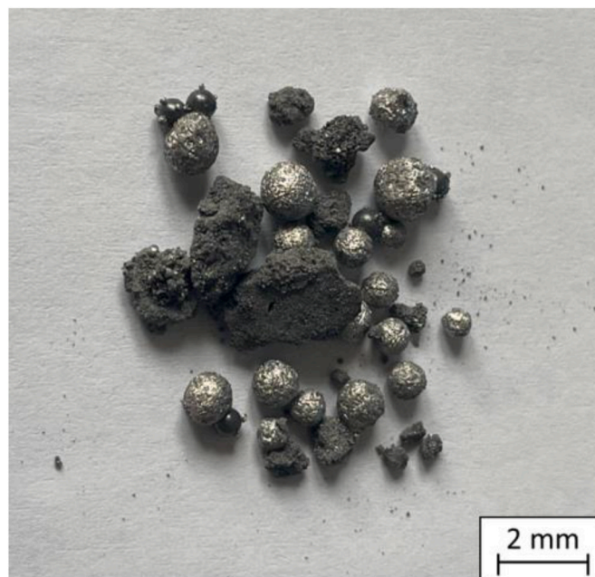
Fig. 2. Steel droplets formed due to carburization of 316 L stainless steel.
