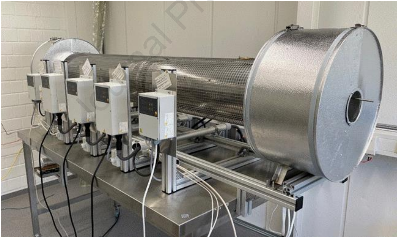
Fig. 2 HoKi furnace dedicated for hydrogenation of 2.5 m long cladding tubes.
