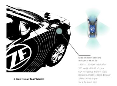
Figure 5.6: Test vehicle for the E Side Mirror application. Displayed on the left is the Hyundai platform, showing the backward-facing side mirror camera, highlighted by the cyan circle (for a more detailed specification of the Sekonix SF3325 [131]. The sensor setup consists of four Sekonix SF3325 cameras. The field of vision of the test vehicle is depicted in the upper right corner as a bird's eye view. The circles represent the camera's mounting position.
