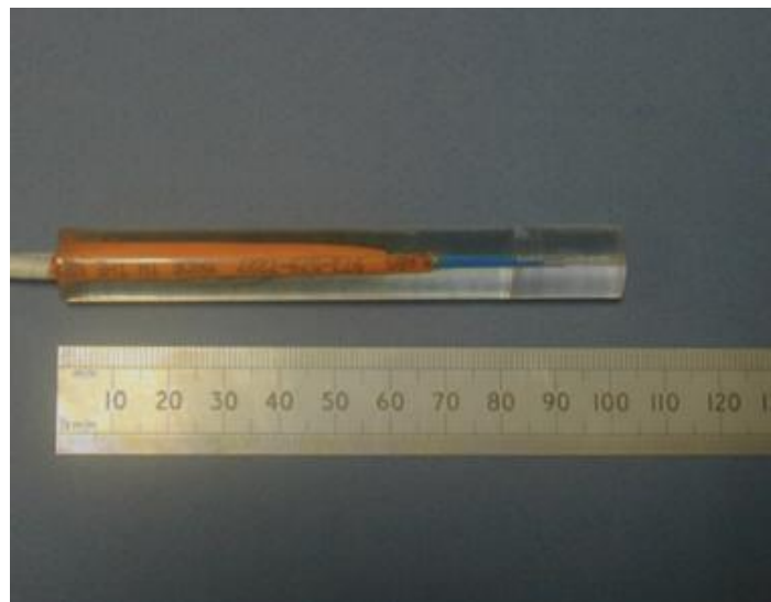
Figure 2.9 - Reflectance fiberoptic splanchnic pulse oximetry sensor
