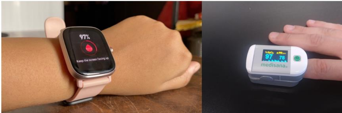
Figure 2.7 - Smart Watch with Reflective Pulse Oximeter (Left) and Transmissive Pulse Oximeter (Right)
