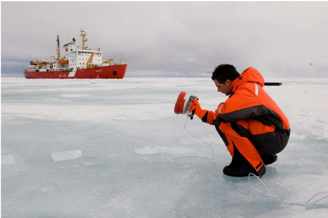
*CO<sub>2</sub> fluxes measurements over sea ice (using chamber of accumulation), CCGS Amundsen in the background*
