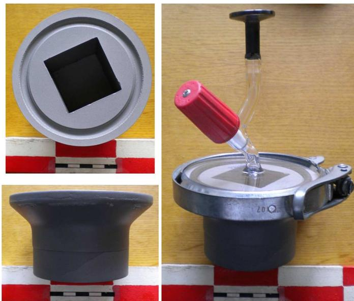
Figure IV.1: Dedicated container for the measurement of pCO<sub>2</sub> in solid sea ice samples, equipped with a flat glass top, silicon joint and a clamp.
