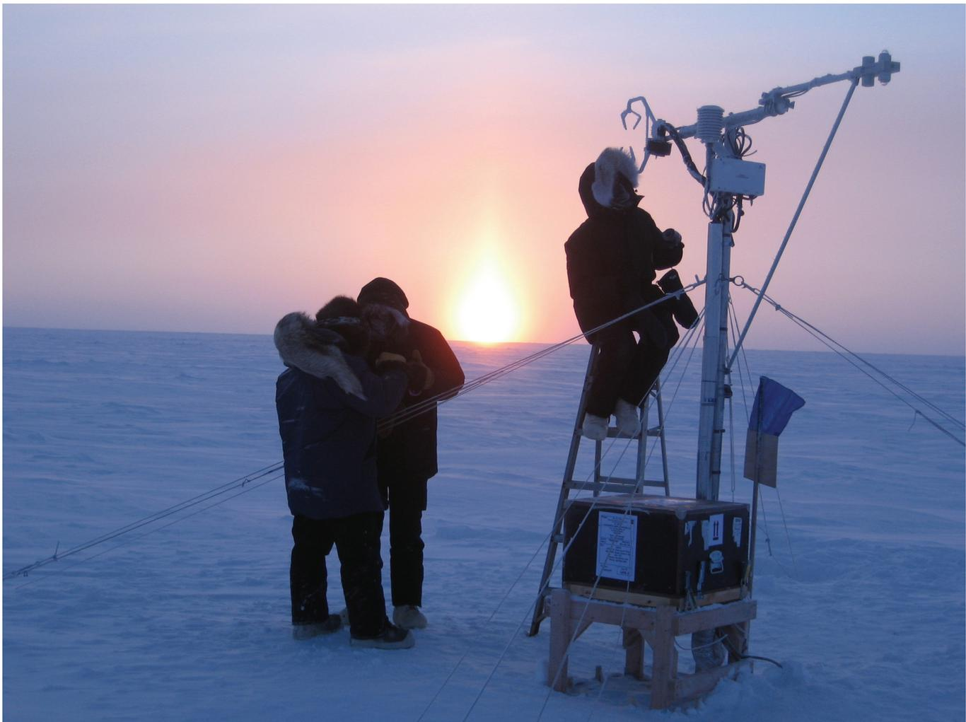
Figure 1: Set up of the mast with sonic anemometer, air intake of the CO<sub>2</sub> analyser and radiometer over sea ice near Barrow (Alaska) in January 2009. The temperature was -35°C.
