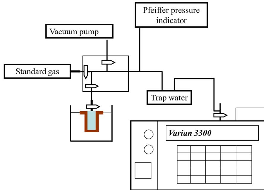
Figure IV.2: Sketch of the different components forming the extraction line, including the Varian 3300<sup>®</sup> gas chromatograph.
