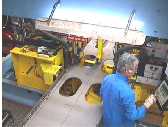
Fig. 14: Fabrication of reconstructed welded profiles
