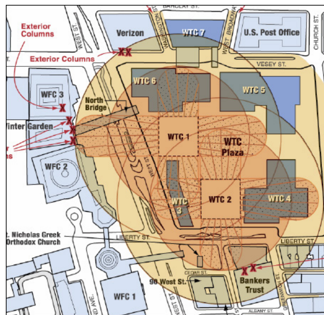
Figure 2.4. A FEMA diagram depicting debris distribution from the collapses of WTC 1 and 2. Dotted, darker and light orange areas denote heaviest, heavy and lighter debris distribution respectively. Red 'X' marks denote isolated perimeter columns ejected farther than in average debris distribution [FEMA, 2002].
