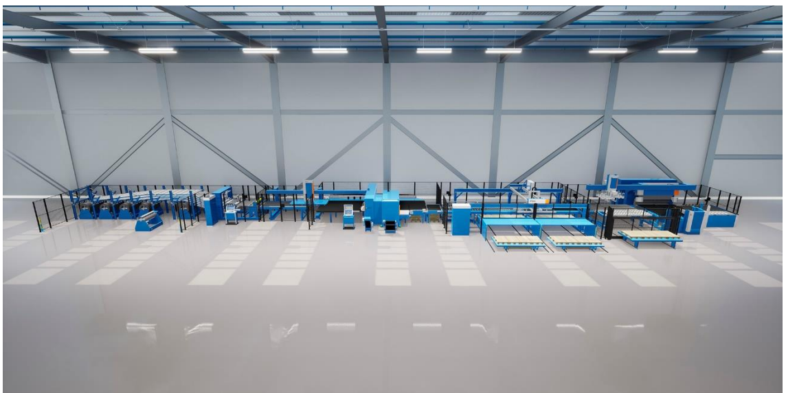
Figure 4: PSBB+ coil line, Prima Power
