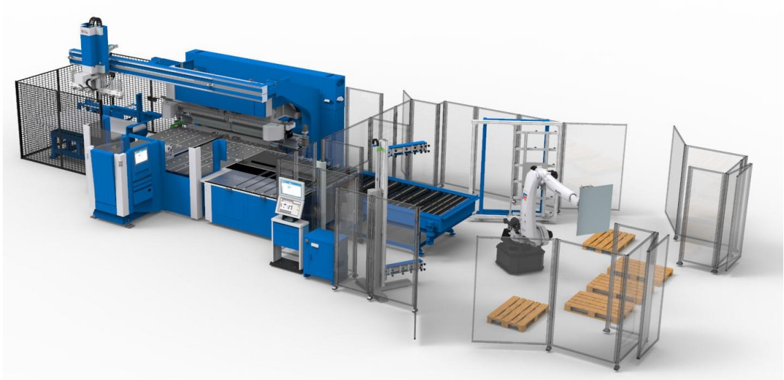
Figure 5: Robot for unloading the finished sheet metal parts, Prima Power
