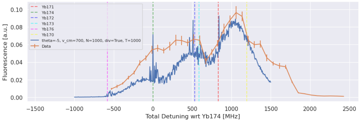
Figure 4.8: Manual fitting with plume divergence spectrum simulation model: A spectrum were simulated with misalignment angles of -5^\circ using the inferred parameters from the low fluence setting pdf. Each data point in the simulated spectra is an aggregate of 1,000 runs. The experimental data were adjusted in both amplitude and frequency offset positioning to show overlap with the simulated results.
