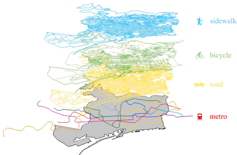
Fig. 6. Multimodal network representation of Barcelona, Spain, with four layers of transport infrastructure (pedestrian, bicycle, road, and metro networks), with data from the Open Data BCN portal for the sidewalk geometries, bicycle paths and metro lines, and OpenStreetMap for the road layer (via OSMnx Boeing, 2017).
