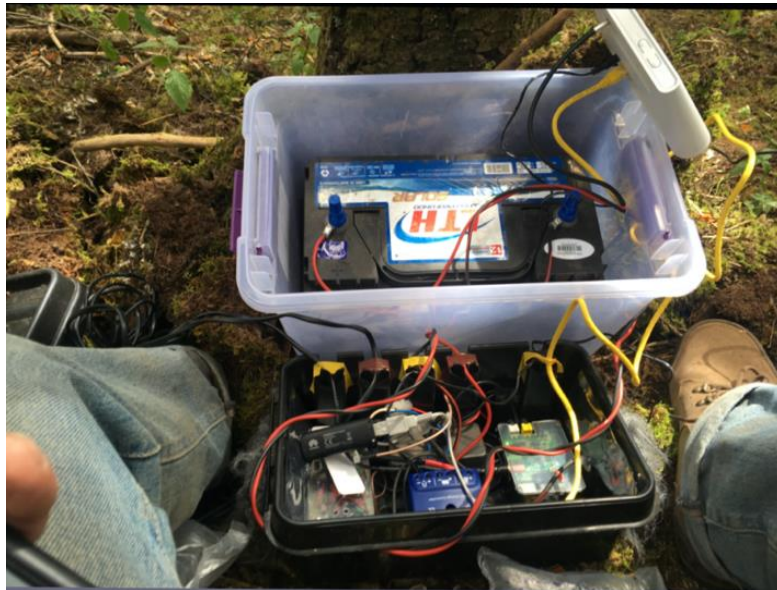
Figure 2. Streambox and battery with wireless router in the Cerro Pelón UNESCO Biosphere Reserve in the State of Mexico.
