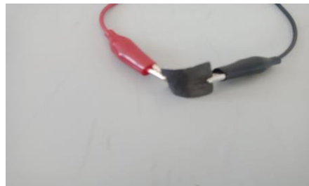
Figure 11. Graphene ink-coated fabric connected with jumper wires
