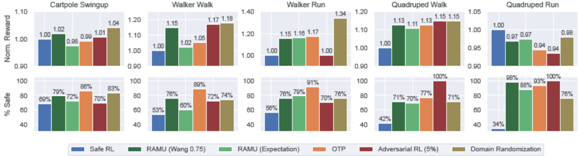
Figure 6-3: Performance summary by task, aggregated across test environments. Performance of adversarial RL is evaluated without adversarial interventions. Top: Average total reward, normalized relative to the average performance of standard safe RL for each test environment. Bottom: Percentage of policies that satisfy the safety constraint across all test environments.
