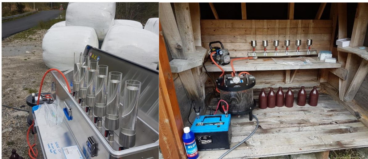
Figure 3 – Vacuum filtration station set-up in the field. A 12-volt battery (80 Ah) was used as power supply.
