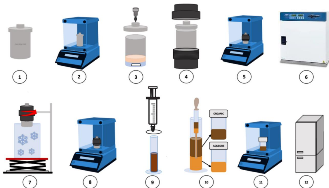
Figure 12: The procedural steps for the conversion reaction of fruit biomass to HMF. Adapted and parts redrawn from Molnes, 2021 72 .
