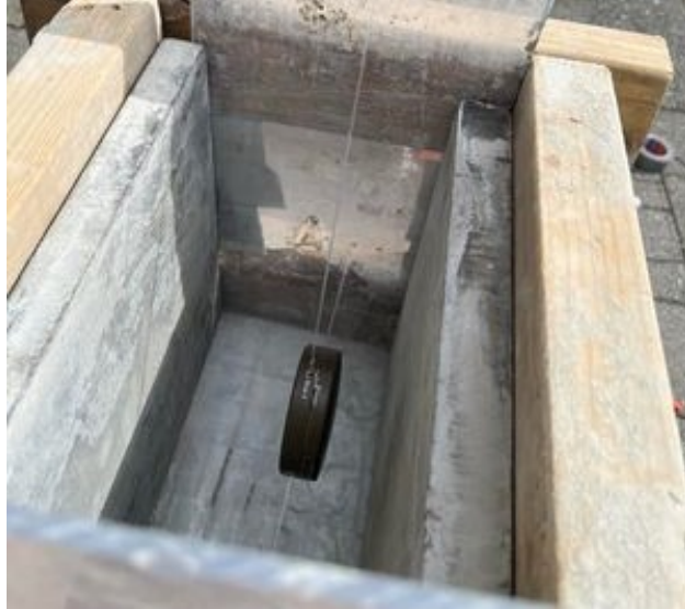
Figure 3.14: How the cylindrical defect was made with a snuff box fastened inside the grout mould at a depth of 5 cm
