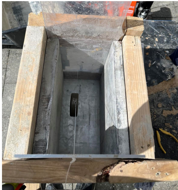
Figure 3.2: Gout mould with cylindrical defect
