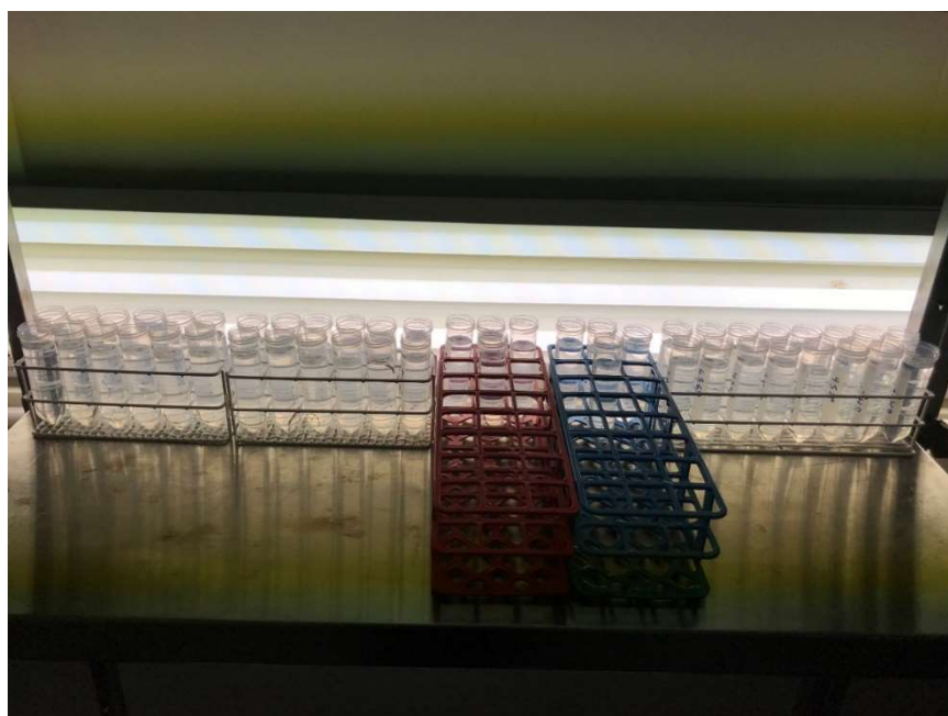
Figure 8 Experimental set up of optimum conditions. Treatment groups and replicates placed randomly. Lamps mounted on the wall behind providing light.
