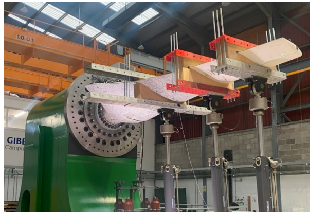
Figure 1. Experimental setup at FastBlade with three saddles clamped to the blade.
