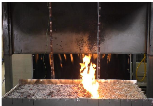
Figure 31. Example of linear flame spread experiments conducted in quiescent, laboratory environment
