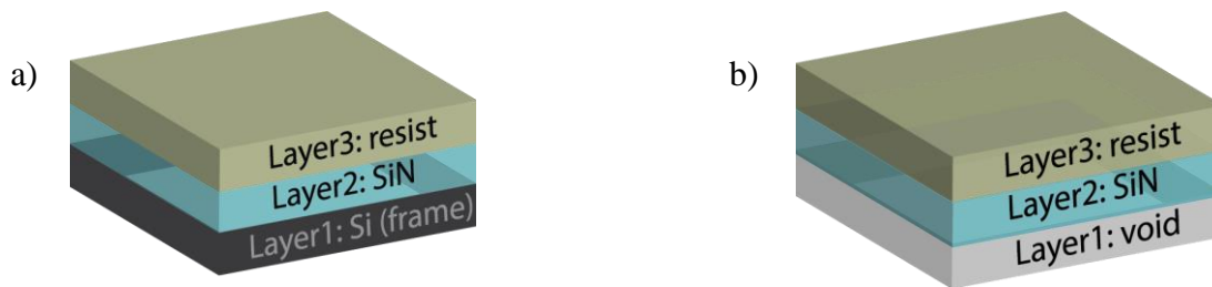
Figure 2.23. Illustration of the models used to fit the ellipsometry data for a) resist on the Si frame of the membrane. b) resist spin coated on top of 30 nm thick membrane.
