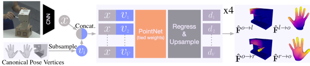
Figure 6. InterField-SF architecture. We concatenate image features \mathbf{x} to each subsampled hand-object vertex in canonical pose. The concatenated vectors are passed through a PointNet and then regressed to distance values. The interaction field is visualized as a heatmap for each entity (bright: closest vertex is near).
