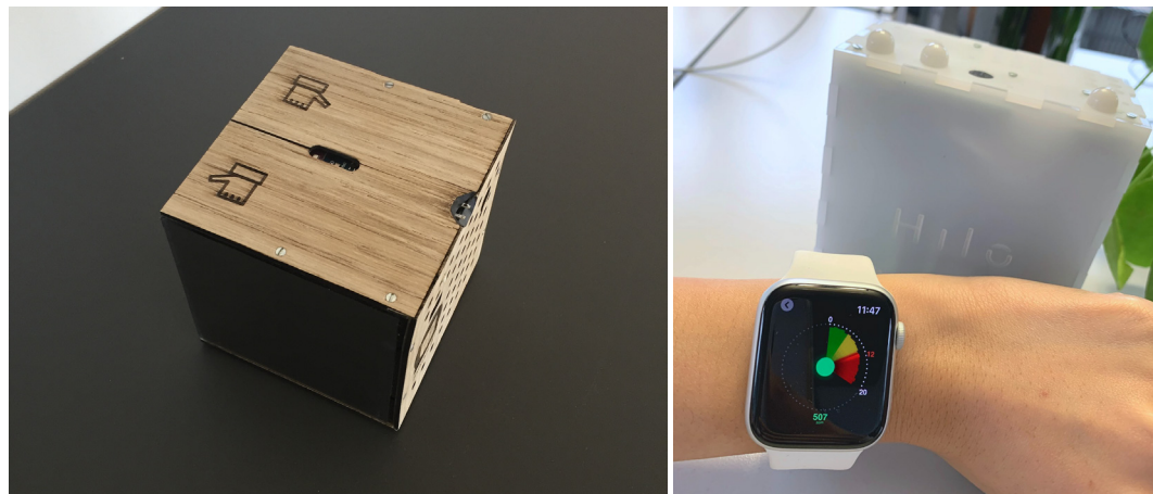
FIGURE 2 Two sensing devices that we developed for recording the concentration of various indoor air pollutants. Connected to these devices, smartwatch and phone applications are provided to make available the live prediction of indoor air quality..
