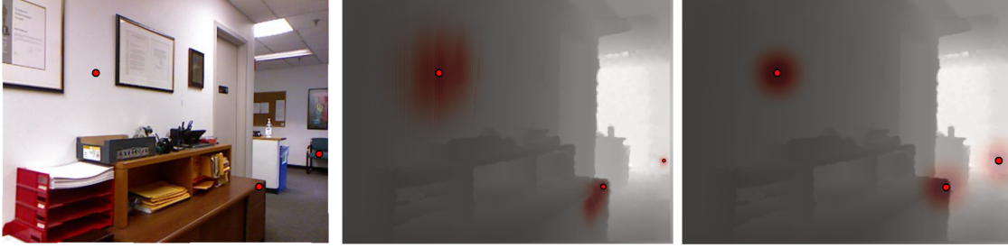
Figure 2. Visualization of the effective receptive fields [22] sampled at three certain points. Left: original image. Middle: effective receptive field of 3DN-Conv. Right: effective receptive field of standard convolution. Results in six sequential layers of 3DN-Convs.
