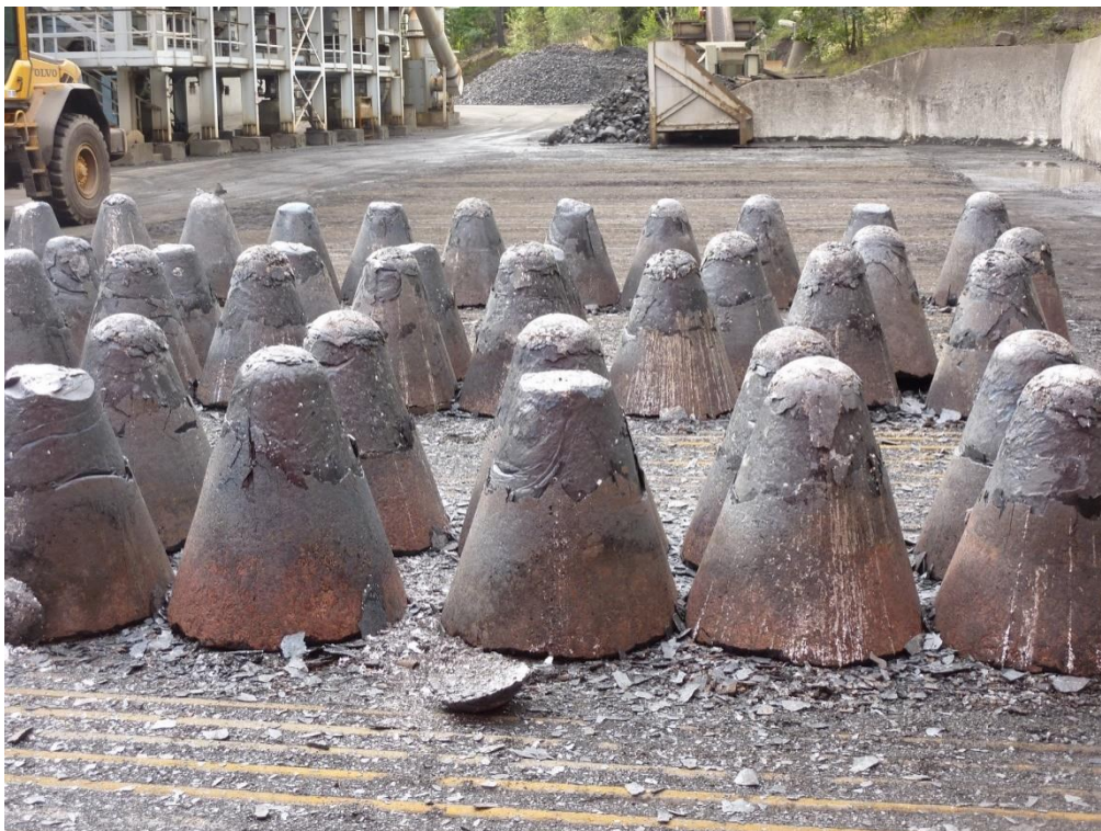
Figure 8. Slag ladle casts after solidification (Secondary Pb smelter, Kovohutě Příbram, Czech Republic; Photo: V. Ettler).
