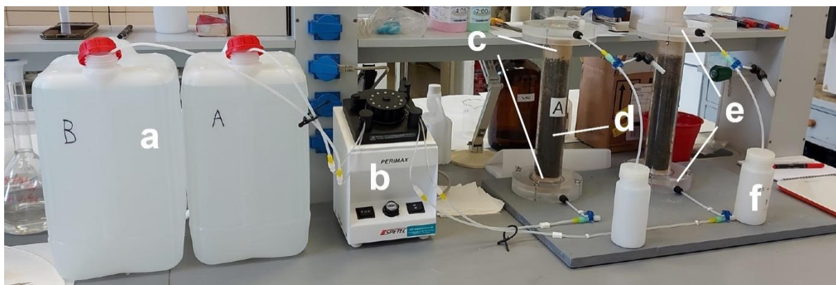
Figure 10. The experimental setup: a) reservoir of the leachant (distilled water), b) volumetric pump, c) layers of quartz sand, d) column with the studied material (Pb metallurgical slag), e) PMMA closings, f) HDPE collection bottle.
