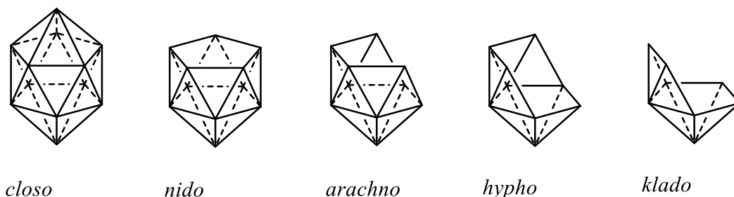
Figure 2.2 Derivation of nido -, arachno -, hypho - and klado -clusters from the original icosahedral closo -cluster according to Wade's rules.
