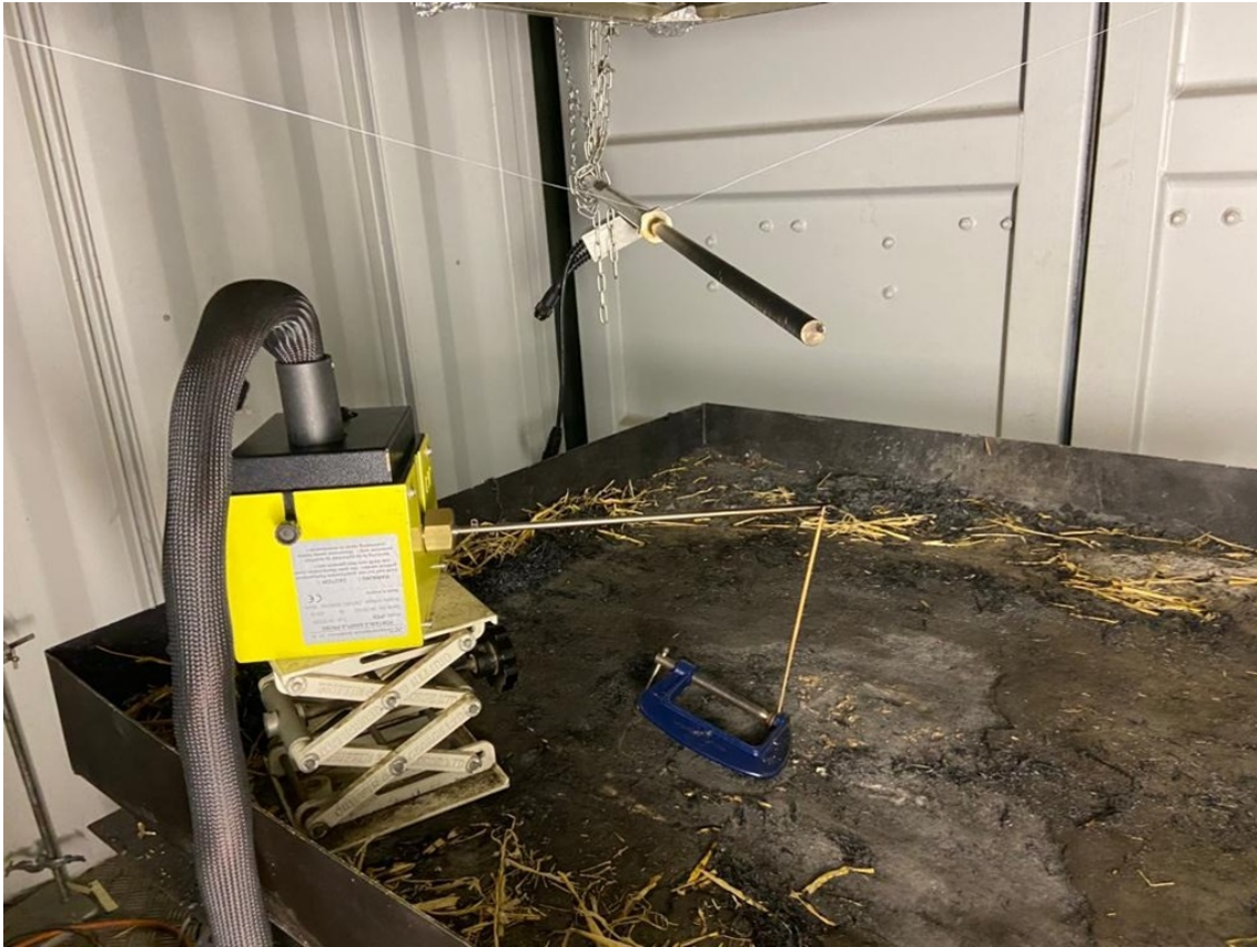
Figure 3.10: Measurement of burning one incense stick on the burning tray.
