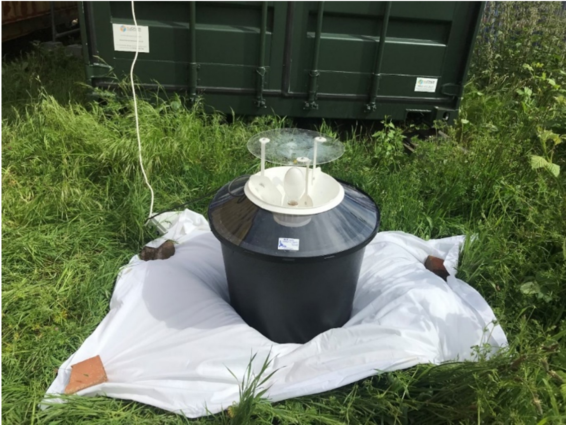
Figure 4.2: A light trap for capturing nocturnal moths. The white sheet is used to reflect the light and increase the overall light intensity.
