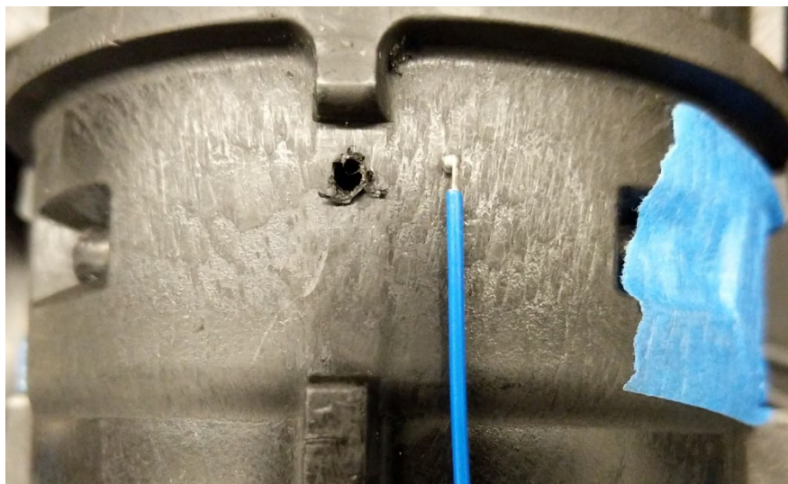
Figure D40: Horizontal method of thermocouple placement
