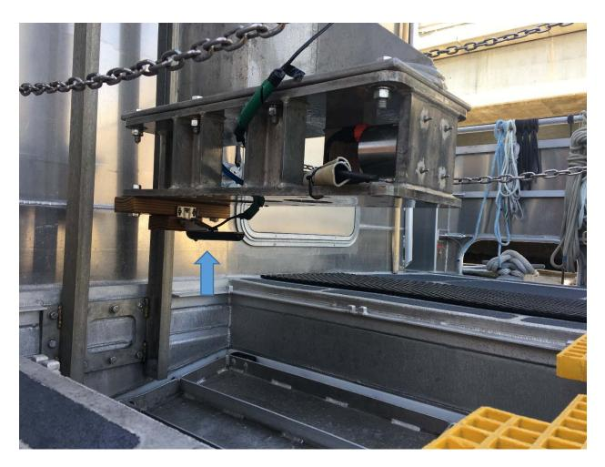
Figure 28: Garmin GT30-TM transducer installed on R/V *Gulf Surveyor's* primary transducer strut. The strut is aligned with the vessel's centerline and can be vertically articulated from the stowed position (shown), to a deployed position which secures the transducer submerged below the hull, clear of bubble wash.
