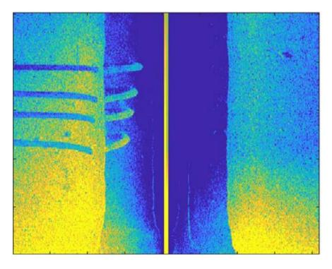
Figure 13: Viz 3 records of full sidescan swath reconstructed using custom MATLAB code. One scanline is composed of 4000 pixels.
