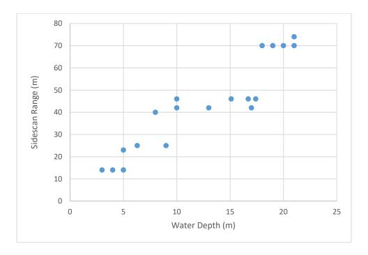
Figure 19: Automatic sidescan range settings applied by the Garmin GCV-10 in water depths between 3-21 meters at 455 kHz CHIRP.
