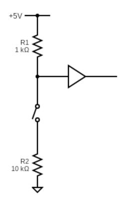
Figure 20: Pull-up resistor circuit diagram. The TCB datalogger utilizes an Odroid C2 computer capable of 5VDC output on Pin 1. Header pin #16 (GPIO #236) registers LOW when the circuit is completed at the transducer.
