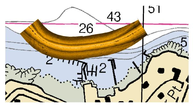
Figure 42: Georeferenced sidescan record collected at 800 kHz with 40m swath width. Overlaid on NOAA chart 13283.
