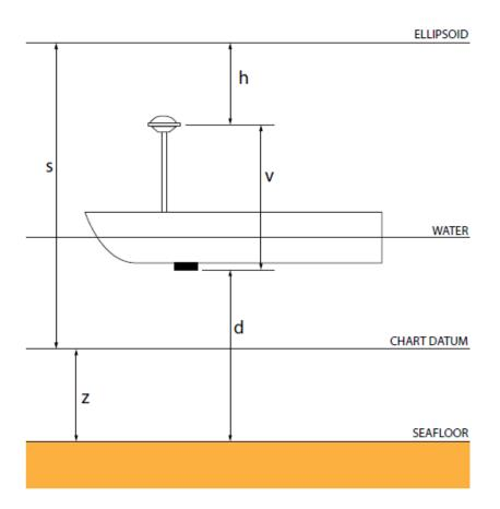
Figure 1: Configuration diagram for static calibration of the vertical offset, v, between the GNSS antenna phase center and echosounder, given knowledge of the depth to datum, z, and the datumellipsoid separation, s. Observed depth, d, and antenna height, h, are measured by the system (Calder et al., 2020). A NOAA tide gauge installed at the adjacent USCG pier measured the water level. (Station ID: 8423898) (Figure from Calder et al., 2020, with permission)
