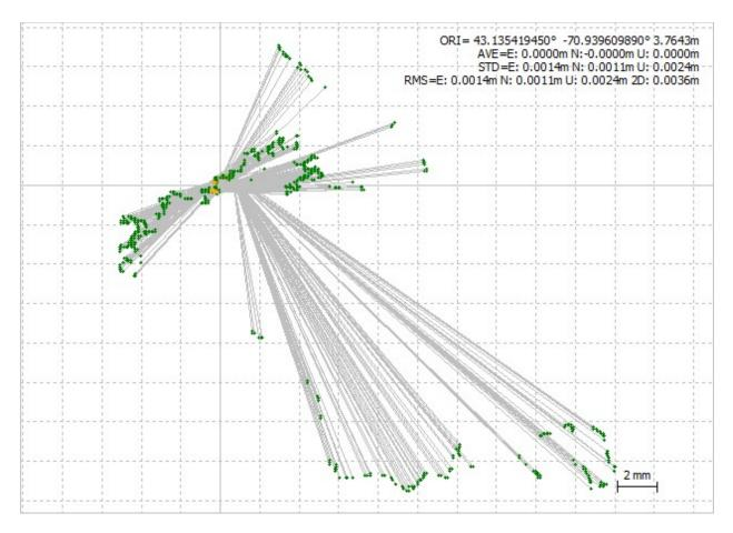
Figure 5: Geographic distribution of post-processed positioning solutions using RTKLIB from 2018-08-09 00:00:00 GPST through 2018-08-09 23:59:59 GPST. Green are fixed ambiguity solutions, yellow are floating point solutions.
