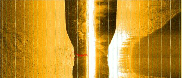
At both test sites, the reported target position did not vary significantly (<1 meter) with vessel speed, indicating system latency has been properly assessed and is not a significant source of positioning error, Figure 33.
