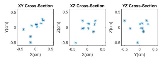
Figure 7: : Two-dimensional cross sections of 10 single point (≈24hr) position solutions from the Harxon GPS500 antenna and SeaID receiver presented in East-North-Up (ENU) Cartesian coordinate system, whereas the East-North (XY) plane is the local horizon plane, and the origin is the average estimated location of the antenna for the entire set of observations. The mean was removed from each axis for simplicity of interpretation.
