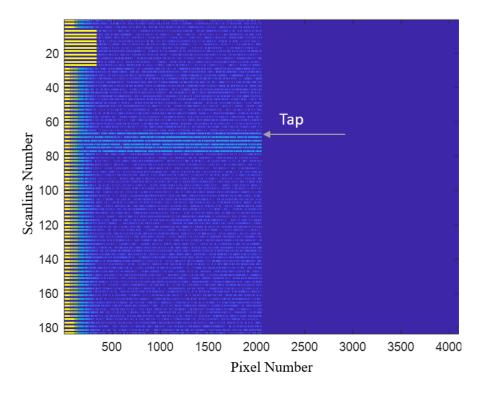
Figure 23: Latency test run at 200-meter sidescan range. Notice the transducer tap is registered as multiple scanlines.
