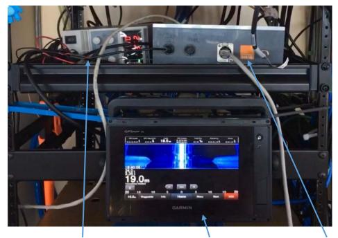
Figure 29: 12VDC Power Supply, Garmin 742XS multifunction display and TCB Datalogger installed on RVGS.
