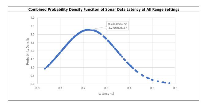
Figure 25: Probability density function of the system latency associated with digitizing Garmin GCV-10 sidescan data and storing it on the TCB datalogger computer. Sidescan range set at 3, 50, 100, 150 and 200 meters. N=257
