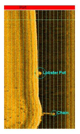
Figure 41: Zoomed in view on two targets visible in Figure 40, with horizontal scale lines at 1 meter interval starting from nadir. Notice the system's ability to image the buoy line coming off the lobster pot, and the mooring chain for USCG navigation buoy GC'3'.
