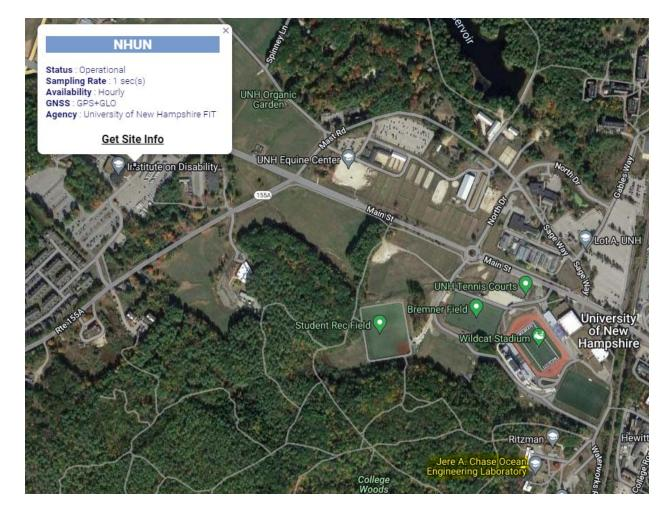
Figure 4: Satellite imagery showing relative locations of NOAA CORS Station (NHUN) and the Jere A. Chase Ocean Engineering Laboratory (highlighted in yellow), where the experiment took place. The baseline distance between the two antenna locations is 1277m. Image taken from NOAA CORS Map online: https://geodesy.noaa.gov/CORS Map/.
