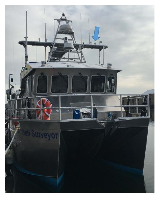
Figure 27: Harxon GPS500 antenna installed on R/V Gulf Surveyor.
