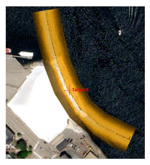
Figure 32: Georeferenced sidescan record with water column removed from latency test site B, overlaid on satellite imagery. Associated sidescan waterfall display, notated with gridlines at 1m interval for scale (bottom). The target position used for the test is notated in both images.
