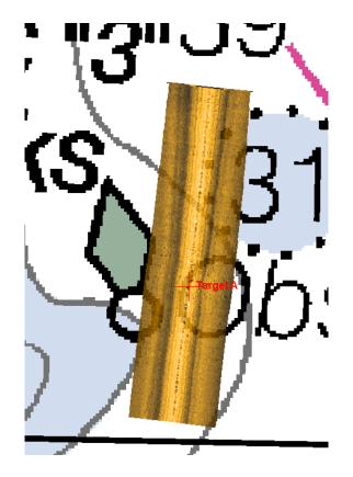
Figure 31: Georeferenced sidescan record with water column removed from latency test site A, overlaid on NOAA chart 13285 (top). Sidescan waterfall display from latency test site A, notated with gridlines at 1m interval for scale (bottom). The target position used for the test is notated in both images.
