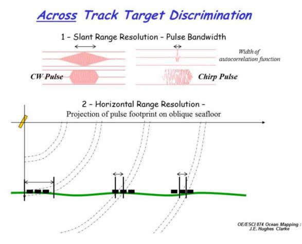
Figure 17: Range resolution model for a sidescan sonar system (Hughes Clarke, 2016). Higher slant range resolution is achieved with physically shorter pulses at a given frequency, or by utilizing chirp pulses which sweep through a band of frequencies, thus dramatically increasing range resolution by decreasing the width of the autocorrelation function. Horizontal range resolution is a function of grazing angle and increases with distance from nadir.
