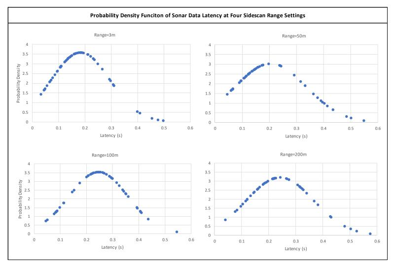
Figure 24: Probability density function of Garmin GCV-10 digitization latency at 3m, 50m, 100m, and 200m sidescan range.
