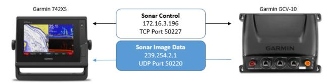
Figure 10: The Control and Image Data streams. Commands for echosounder control are sent to the GCV-10 processor at static IP address 172.16.3.196 on port 50227. The echosounder image data is broadcasted on UDP multicast address 239.254.2.1 to port 50220.
