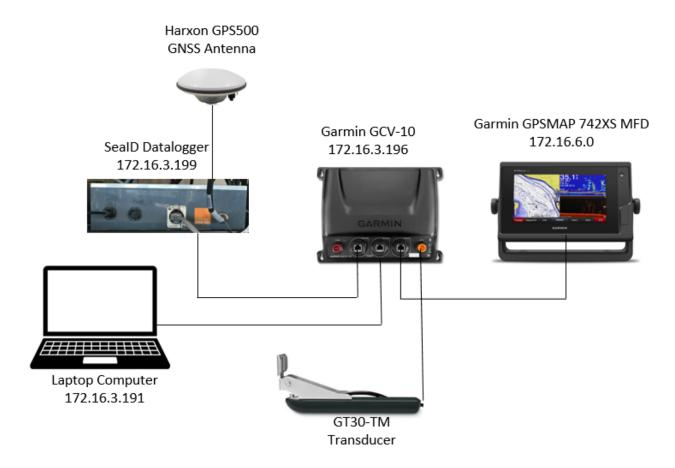
Figure 26: Hardware installation topology.
