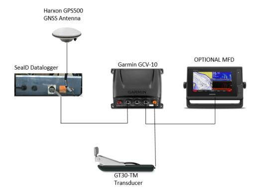
Figure 15: Physical installation schematic for logging sidescan data using the SeaID prototype TCB datalogger. The Garmin MFD is optional because the echosounder can be controlled solely with the TCB Datalogger if there is no need for a real-time data display.
