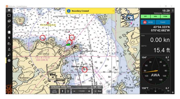
Figure 36: Four boundary circles (red) displayed on *R/V Gulf Surveyor's* chart plotter running Rose Point Coastal Explorer software, marking demonstration targets of interest.
