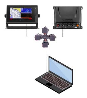
Figure 9: Wiring schematic for passively sniffing network traffic between the echosounder processor and chart plotter using a Throwing Star LAN Tap and a laptop running Wireshark.
