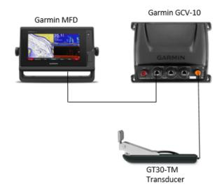
Figure 8: Generic Garmin GCV-10 installation schematic.
