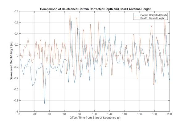
Figure 2: Comparison of Garmin observed depths and SeaID data logger (SDL) antenna heights, demonstrating that the motion effects are captured in the antenna height to some extent as well as in the depths, and that there is a significant latency in the timestamps associated with the Garmin observations logged by the SDL. Note that the means have been removed from both signals to allow for plotting on the same scale (Figure from Calder et al., 2020, with permission).
